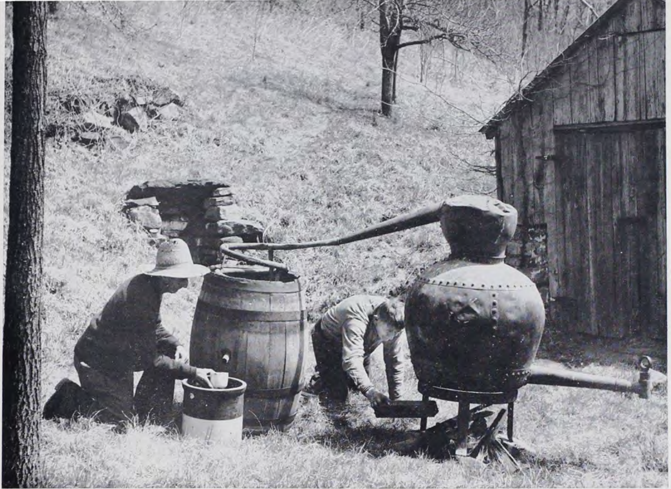
An early 19th Century Pennsylvania Dutch still made entirely of copper—found in the hills near Kutztown. Notice the tank spigot to clean the 50-gallon boiler. From the author's collection.
