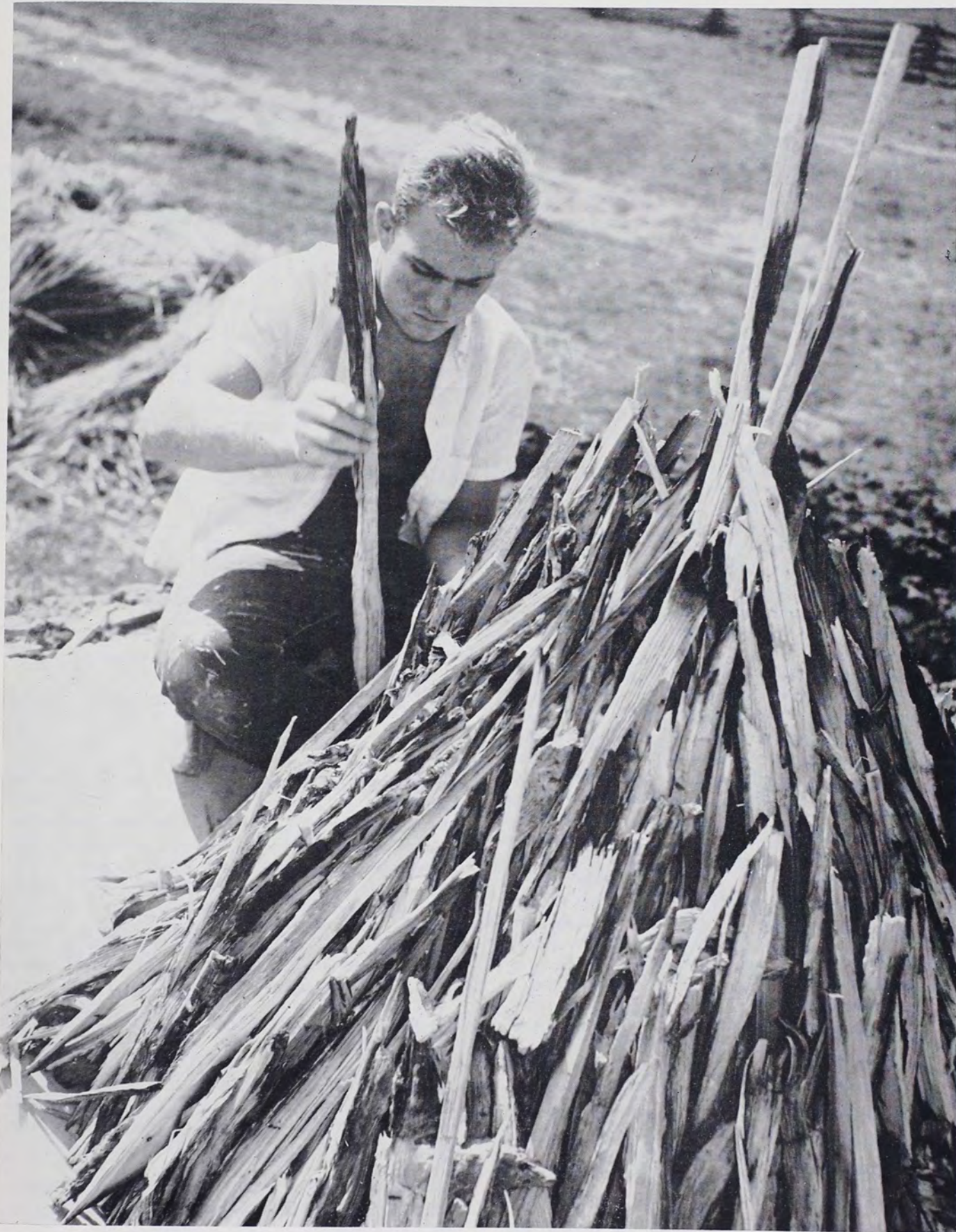
Building the pyramid of pine kindling out of which pine tar is extracted. Faggots are covered with wet straw and clay, then set on fire to burn slowly for several days.
