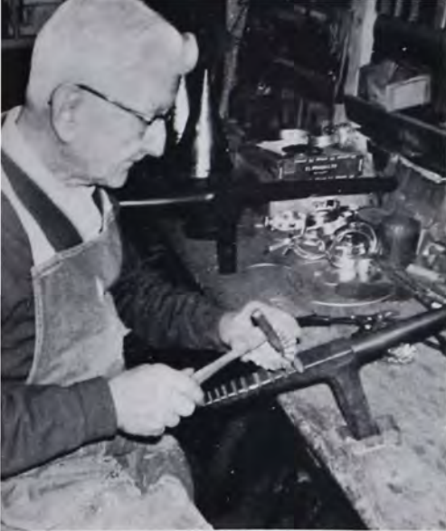
Using the creasing stake to make drip-catcher for chandelier.
