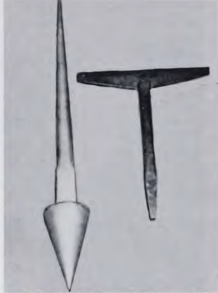
Tools of the tinsmith trade: Blow-born stake and Hatchet stake.
