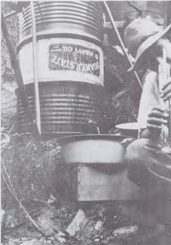
Fig. 5. Fleegal checks the proof of the whiskey coming from his condenser.
