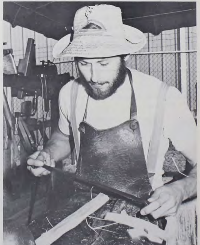
The author uses his drawknife while holding the piece of wood with the "schnitzelbank".
