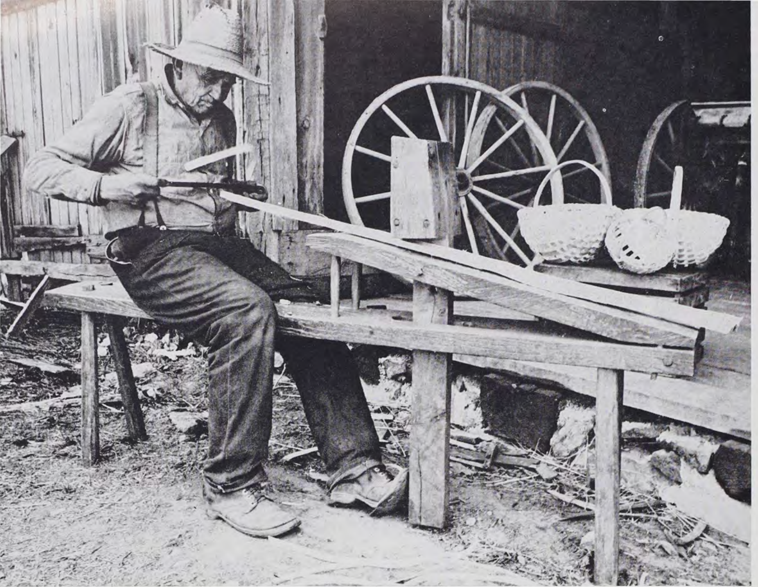
Picture B—Shaving smooth a rough split of wood on the shnitzel-bunk , so that it may be made into rims and handles for baskets.
