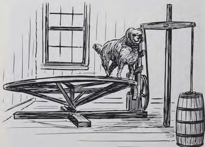
Dog-power treadmill for churning. Note barrel churn at right. There were many patented models in Victorian days.
