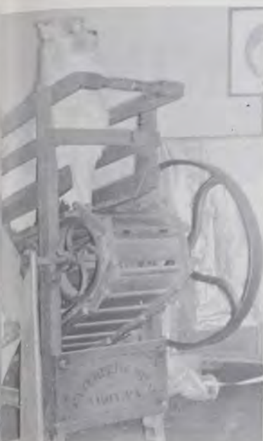
Dog-Churn patented 1881 by the Enterprise Manufacturing Company, Troy, Pennsylvania. Photograph by George G. Miller.
