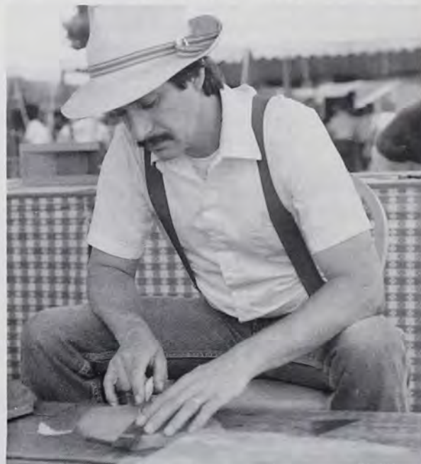
The author is shown scribing the hour lines on one of his flagstone sundials.
