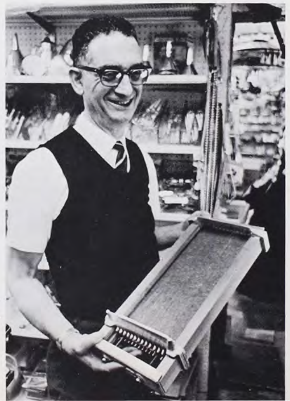
The machine is called a "guitar" by Italians and is used for making pasta.
