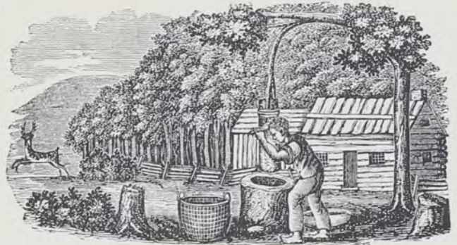
Before gristmills were erected in the early settlements, the pioneer farmers used primitive methods of pounding grain. This picture, from Sherman Day's Historical Collections of the State of Pennsylvania (Philadelphia, 1843), shows a corn mill made of a hollowed-out stump, with the pounder attached to a flexible tree limb. The apparatus was known as a "hominy mill".
