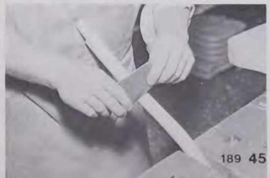
The author scrapes the bent back piece to a smooth finish, before drilling spindle holes.
