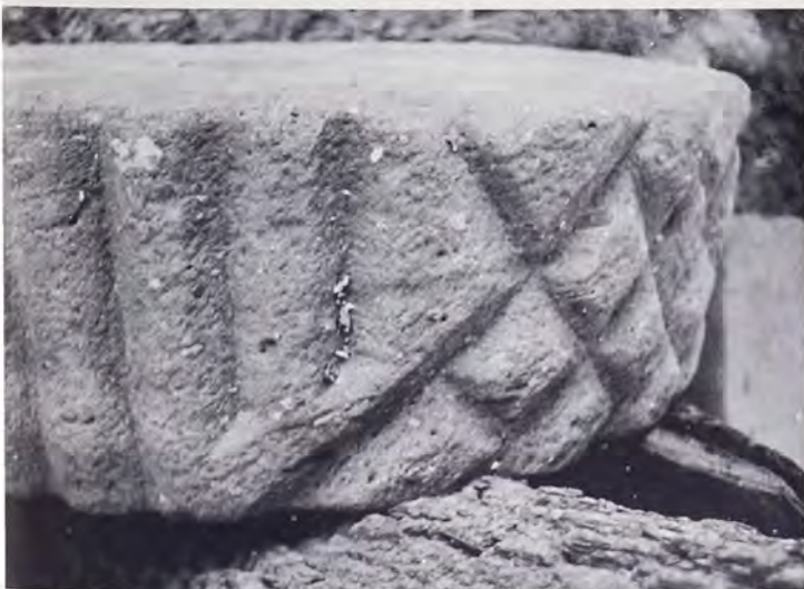
Bark Mill-Stone used in Bark Mill to prepare bark for tannery use. Note the two types of incision on the stone face; the intention was to shred the bark rather than pulverize it, thus retaining the tannin qualities in the shredded bark. For position of stone in bark mill, see plate on page 10. Collections of the Chester County Historical Society.
