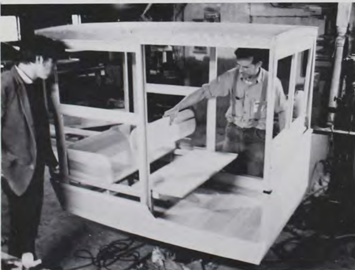
Front seat is now in place, ready for upholstering.
