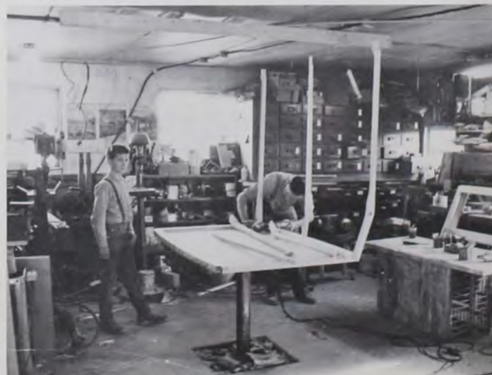
Adding the upright supports to the coach. Their number gives the Mennonite Carriage its local name, the "Six-Poster".
