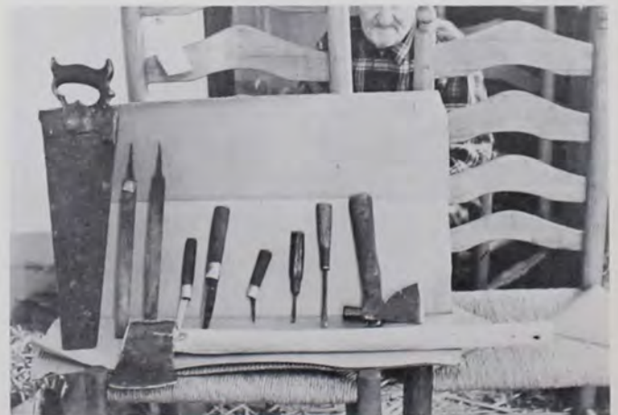
Tools. Left to right: (1) saw, (2) coarse and fine rasps, (3) knives, (4) chisels, and (5) hatchet and axe.
