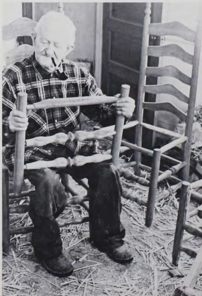
Assembling understructure of chair.
