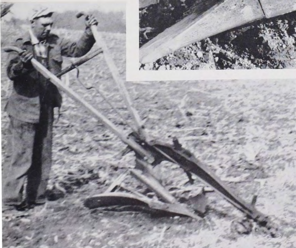
Tumbling the hillside plow to change it from a right- hand to a left-hand plow, or vice versa. Note adjuster be- tween handles.
