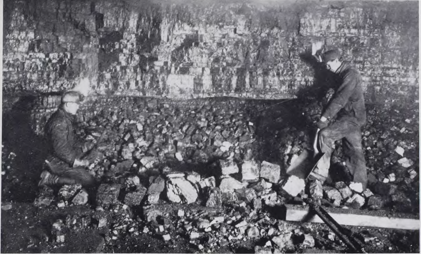
Once in the mine the miner operates in a world of semi-darkness, attempting to extract as much "black gold" as possible during his shift. Here, two miners stand by a "breast" of coal which is ready to be shoveled into waiting coal cars for shipment to the surface and the coal breaker.
