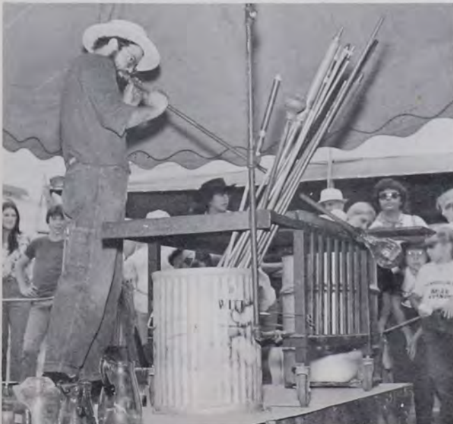
A bubble of glass is blown with the pipe until the desired size is reached.
