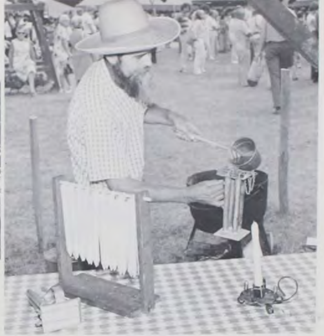
Abe Stauffer pours tallow into tin candle moulds, demonstrating another method of candle making.
