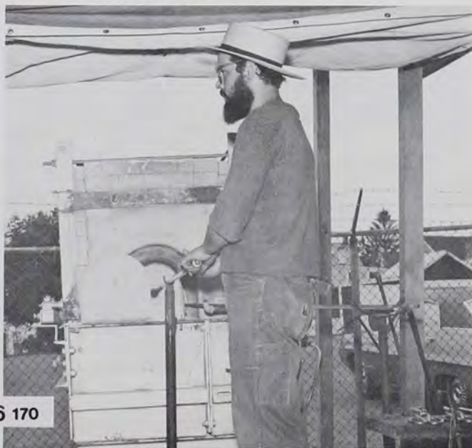
The glassblower picks up, with the pipe, a molten blob of glass.
