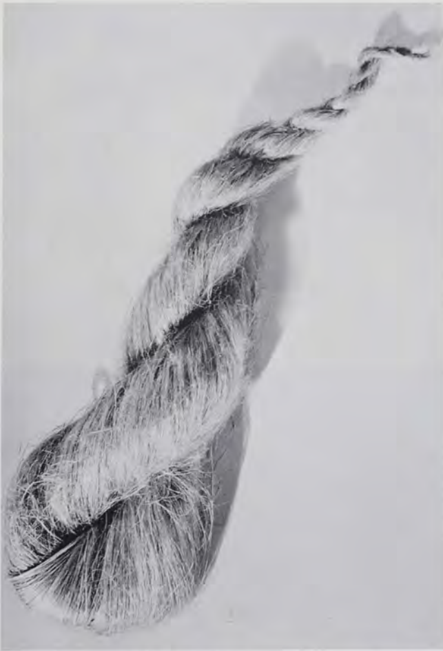
A single flax strick ready for storage prior to spinning showing the tight even twist.
