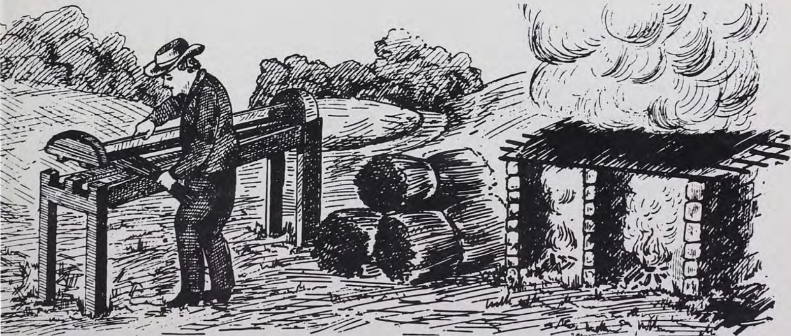
This old cut shows the brechloch with the flax kiln, bundles of retted unbroken flax and the flax brake in operation. (From Eli Keller's Flax and Its Utility ).
