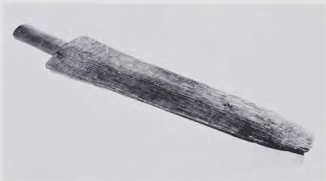
Double-edged scutching knives of this kind were commonly used throughout most of Pennsylvania.
