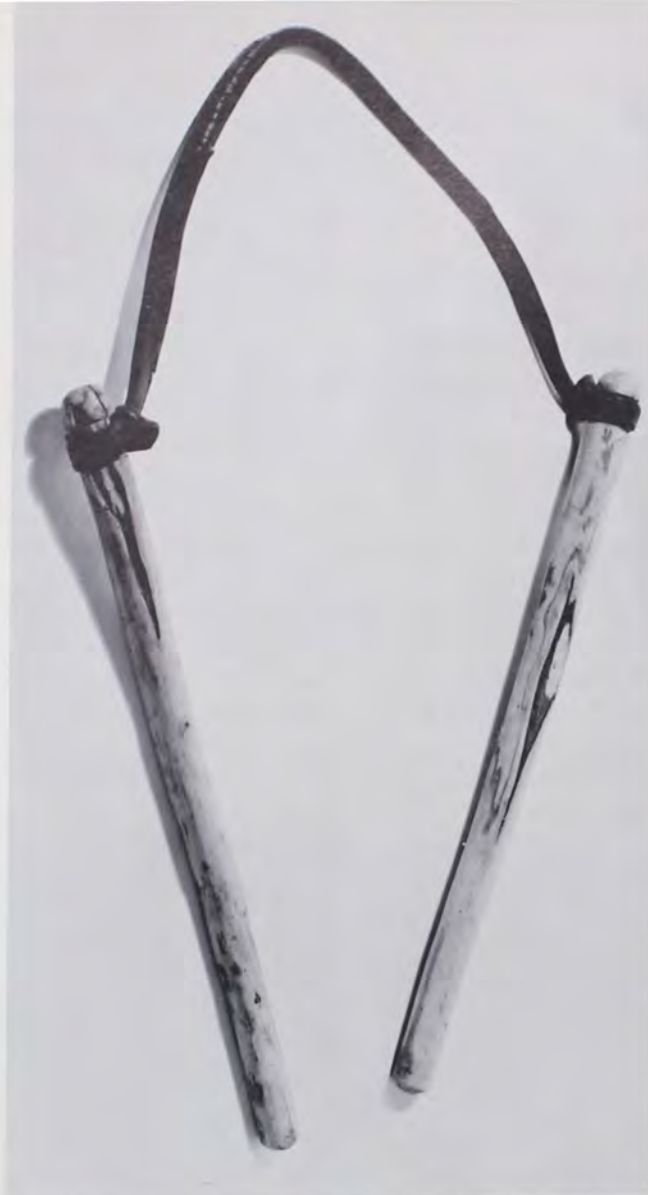
The flachsgnewwel was used as a clamp to hold the handful of flax during the braking process. Courtesy of the Schwenkfelder Museum, Pennsburg.
