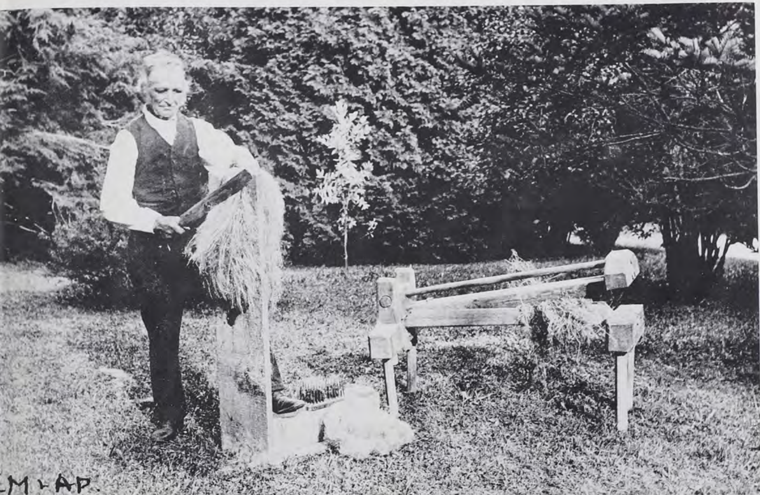
An old man photographed scutching flax at the close of the 19th Century. Courtesy of the Mercer Museum, Doylestown.
