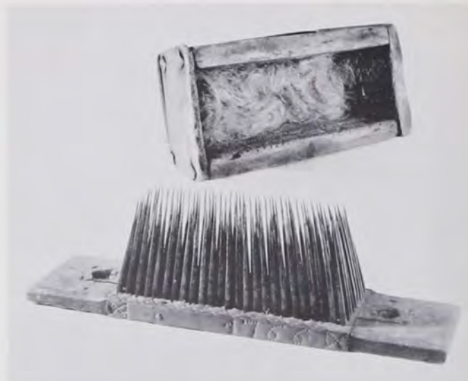
Most flax hackles originally had a wooden cover. Here the cover is shown with the old tow wad in the lid to protect the iron spikes. Courtesy of the Goschenhoppen Historians Museum, Green Lane.
