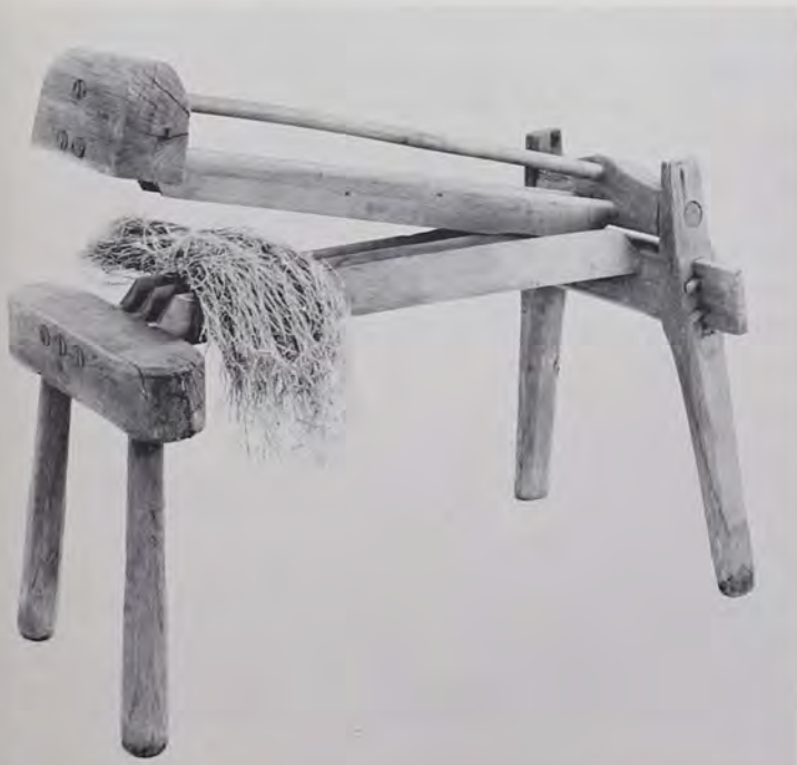
This type of flax brake was the one most commonly used in Pennsylvania.
