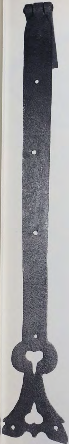
An extremely venerable strap-hinge. The method of creating a heart by means of contiguous circles elongated to form a point is clear in this medium.
