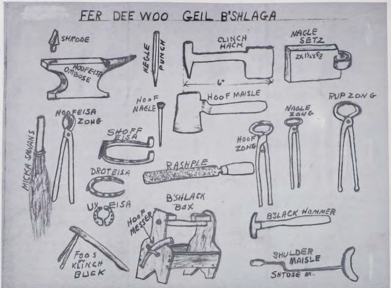
Tools used by the blacksmith to shoe horses, drawn by the author.
