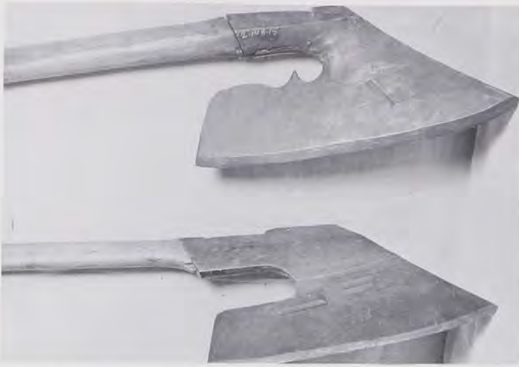
Short-handled "goose wing" axes like these were used to hew timbers for the Herr house. (Private collection)
