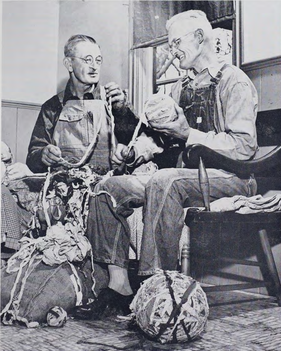
After the strips are sewed, they are rolled onto balls. Allen Stephen and Martin Wetzel show how it's done. The balls were put in bags and were then ready for delivery to the local carpet weaver.
