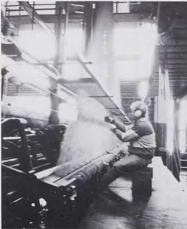
Technician tying the harness of a loom at the Scranton Lace Co.
