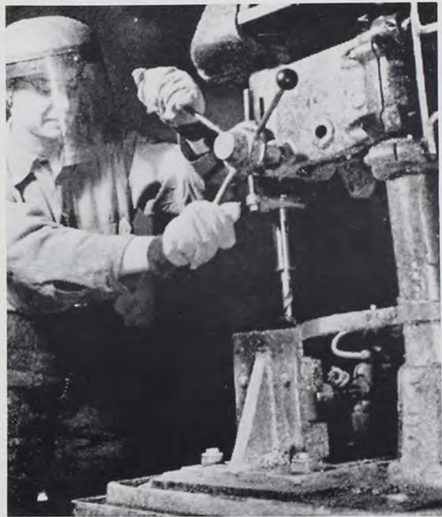
During World War II many women took jobs that had traditionally been considered "men's work"; this woman is boring tong-holds in freshly cut aluminum alloy stock for making forgings.
