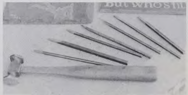
These are the chisels and hammer used by the author, to hand cut his metal and slate engravings and dies.
