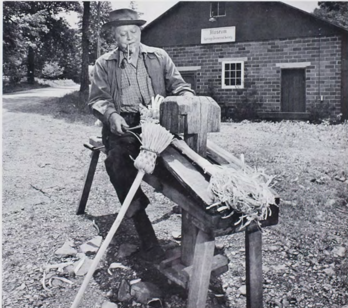
Claude ("Simps") Miller Shaving Hickory Brooms on a Shaving Horse or "Schnitzel-bank."
