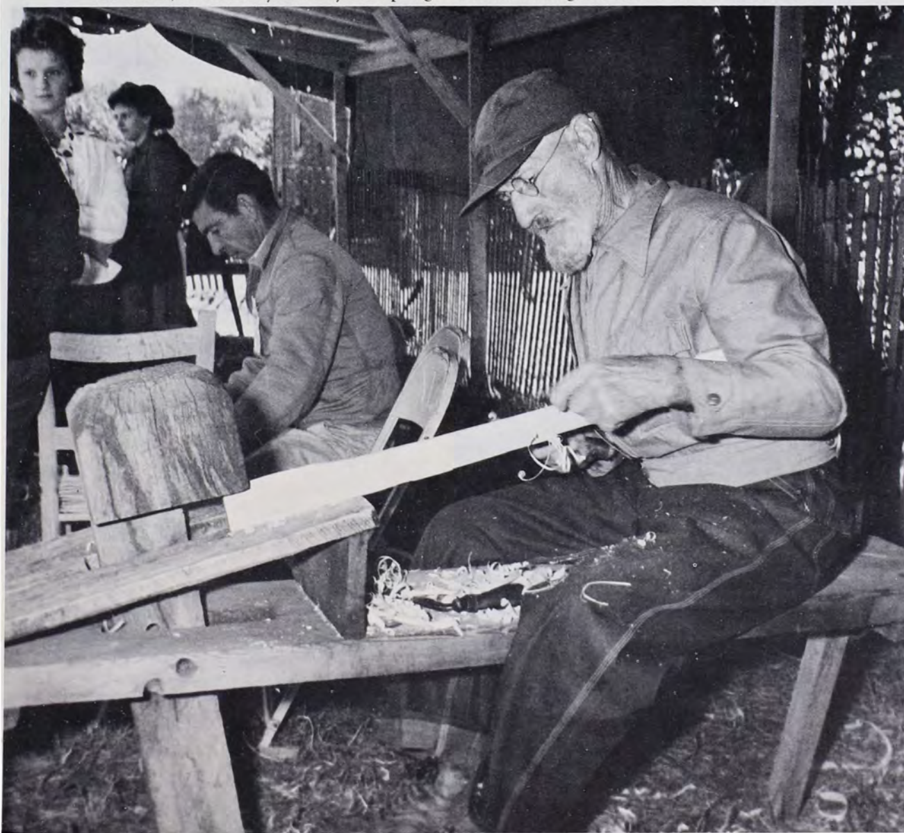
Ad Maust, Senior Craftsman of the Springs Festival, making axe handle on a schnitzelbank.
