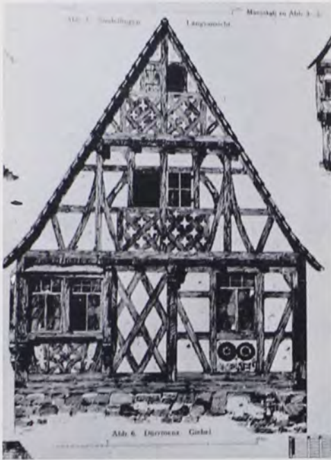
Half-timbered steep-roofed farm housing in South German village of Dürrmenz. Note secondary angle of roof-pitch (kick) just at the eaves, like Swiss counterparts.
