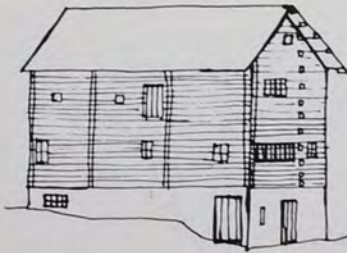
Pure log construction of the Northalpine Region built prior to 1417, in Flüeli near Sachseln (after Weiss - illus. 9 - "Häuser und Landschaften der Schweiz." Birthplace of Brother Klaus
