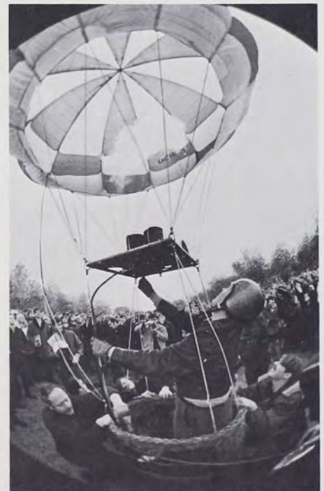
While the crew restrains balloon, final adjustments of temperature within balloon are made, varying between 150 and 200 degrees above unheated air. Photo by James Baird with Fisheye lens.
