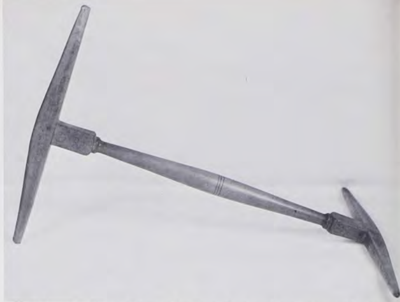
A well worn niddy noddy, or hand winder for skeining yarn. The initials D. R. indicated the owner.
