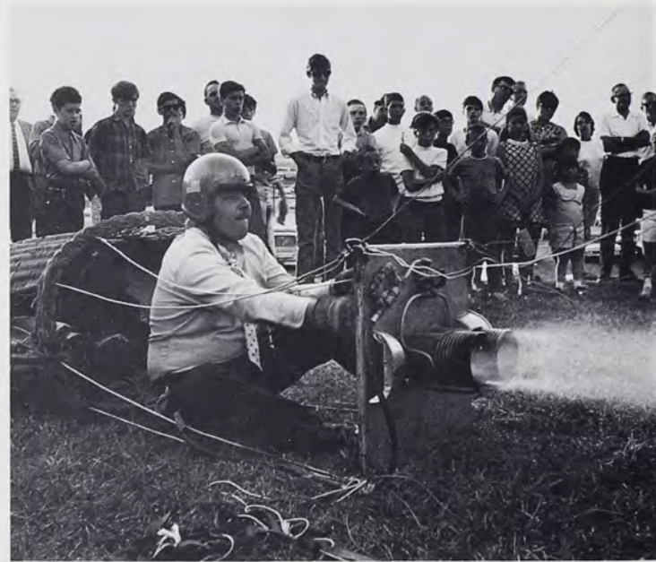
Burner tubes turn white as water freezes on them from cooling effect of expanding propane as air is heated to inflate the balloon.
