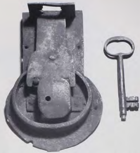
Chest lock with key. These were known as “grab” locks. (Author’s Collection)
