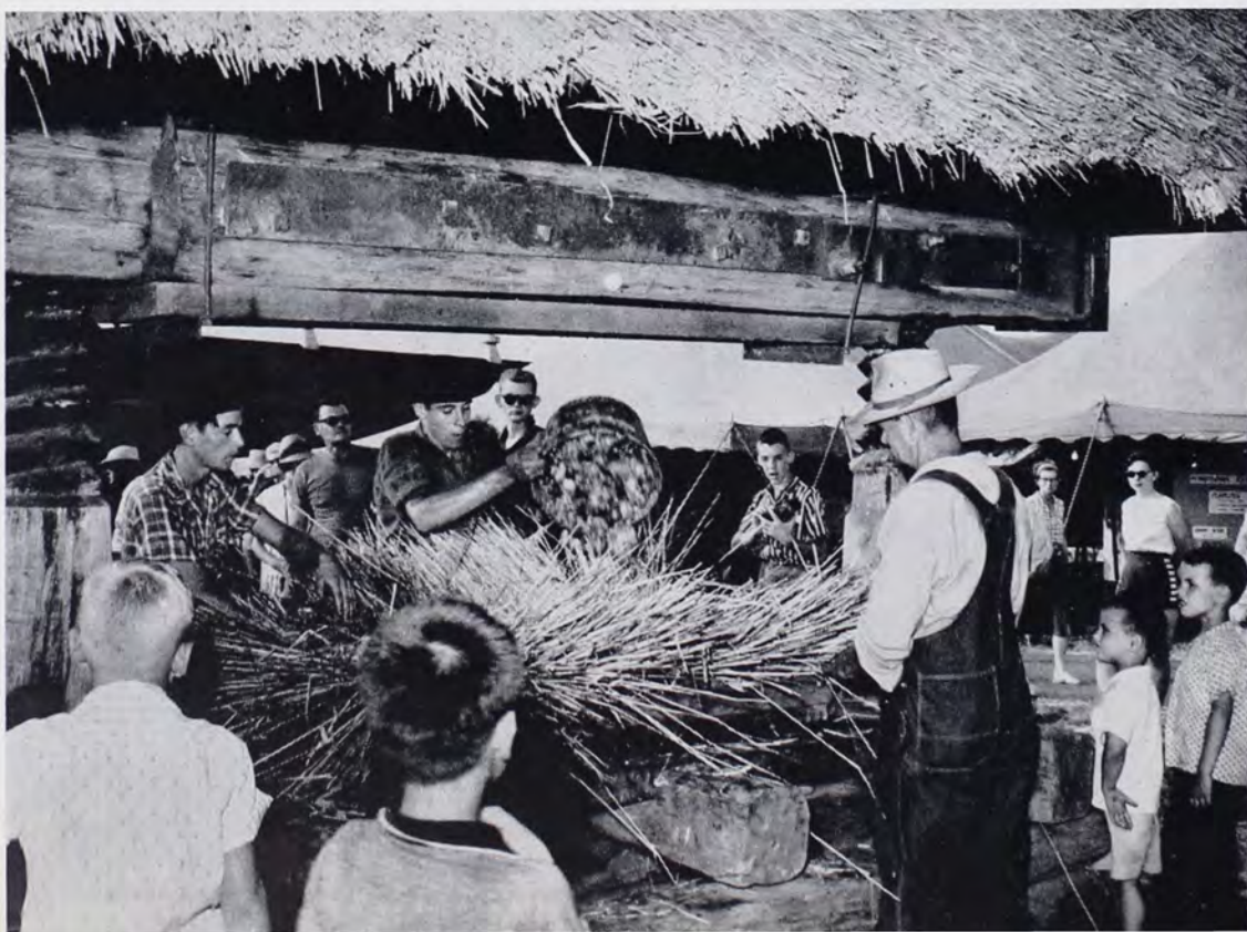
18th Century Cider Press Demonstrated at Festival—Ground Apples Are Placed on Bed of Straw in Preparation for Pressing.
