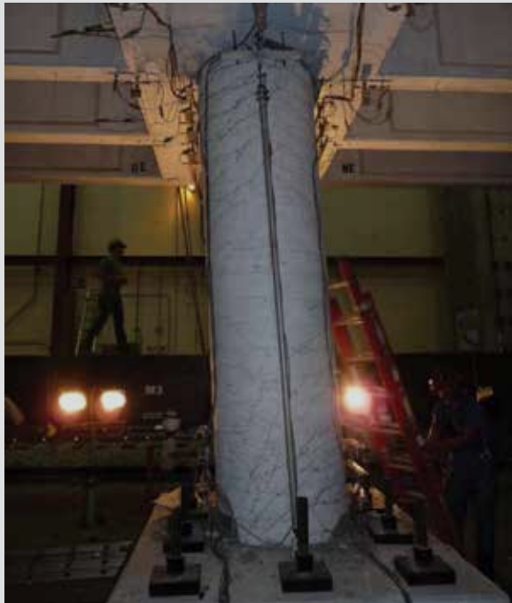
Column at 7 in. lateral displacement (displacement ductility +10.0)
