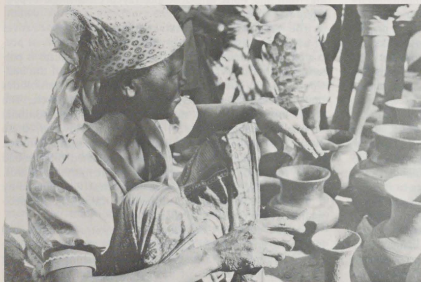
Figure 5 —A corncob is used to shape the surface of the pot, which is turned slowly by hand without a potter's wheel.
