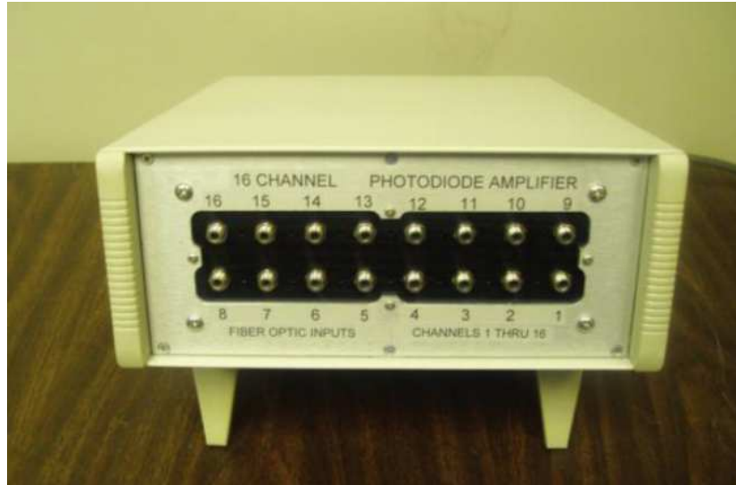
Figure 4.29: In-house built dosimetry system to measure fluence
