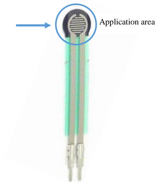
Figure 7: FSR application area is highly sensitive. If the distribution of force moves around on the application area, the output changes drastically.
