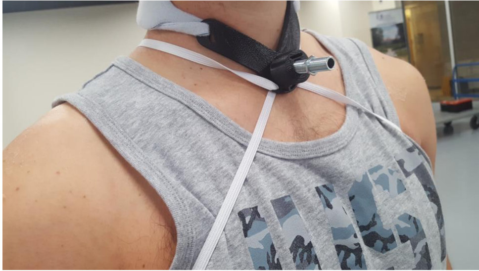
Figure D1: Two straps hold the device in place. The top strap secures the device to the neck while the bottom strap pulls the device into the tracheal region.
