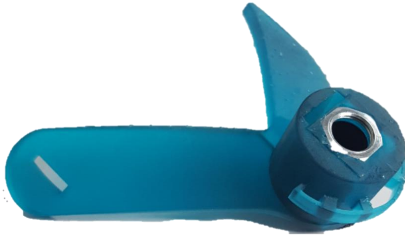
Figure 12: Final prototype printed using tough resin; this material is stronger and more comfortable for the user
