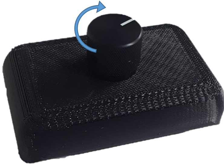
Figure 14: The potentiometer controller was placed in a box to keep all wires away from the user and give the user a firm box to hold on to. The knob allows the user to easily adjust and click off the vibration frequency.
