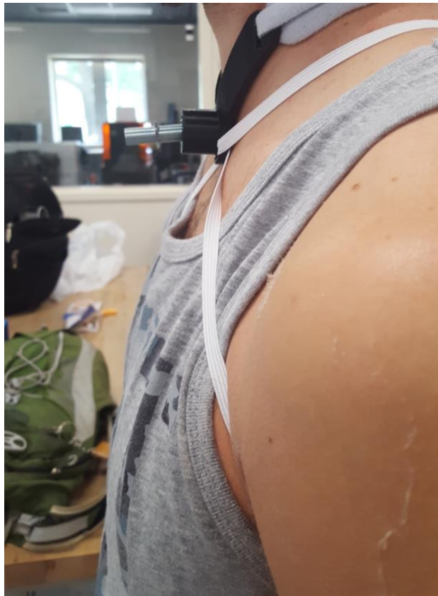
Figure D2: Side view of device being worn with two straps; the bottom strap is flush with neck, which was later changed to improve the pull towards the tracheal region of the neck
