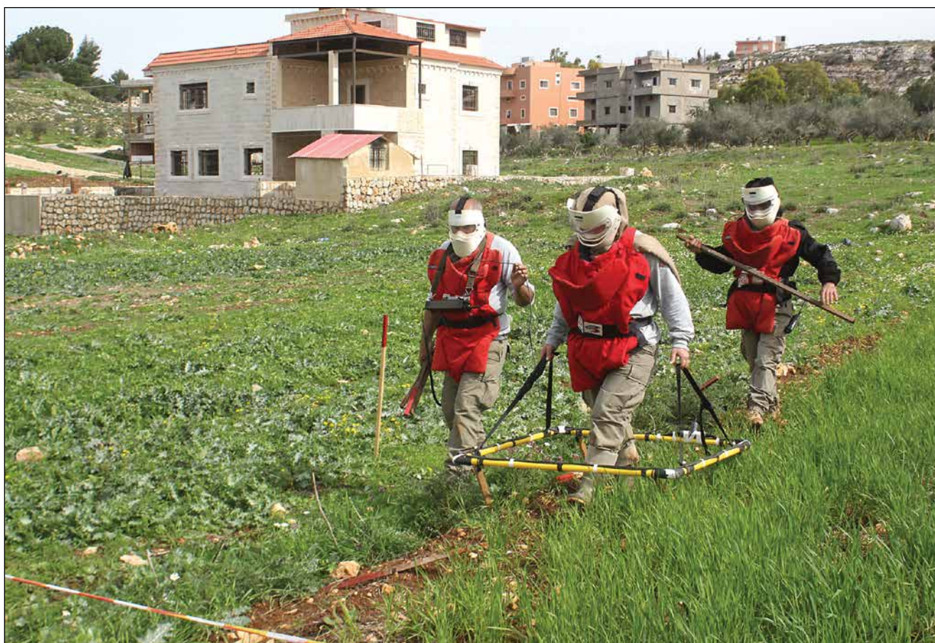
DCA deminers, funded by PM/WRA, use a large loop detector to conduct sub-surface clearance in Lebanon. Photo courtesy of DCA.
