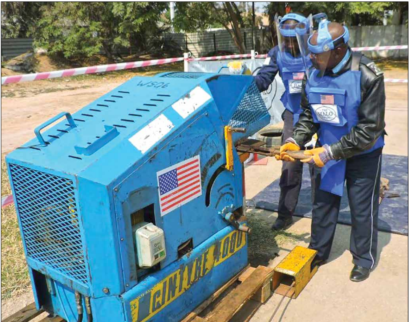
A HALO weapons and ammunition destruction team funded by PM/WRA in Benguela, Angola, cuts state-held weapons to render them useless. Photo courtesy of HALO.
