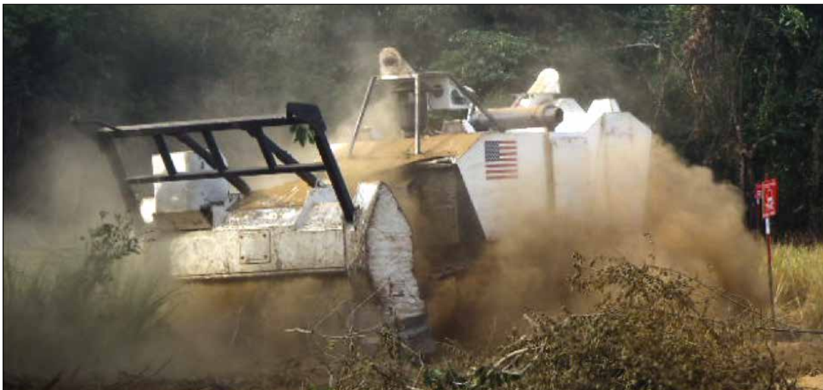
MAG uses the HD R&D's Mini MineWolf to clear a minefield in Cambodia. Photo courtesy of MAG.
