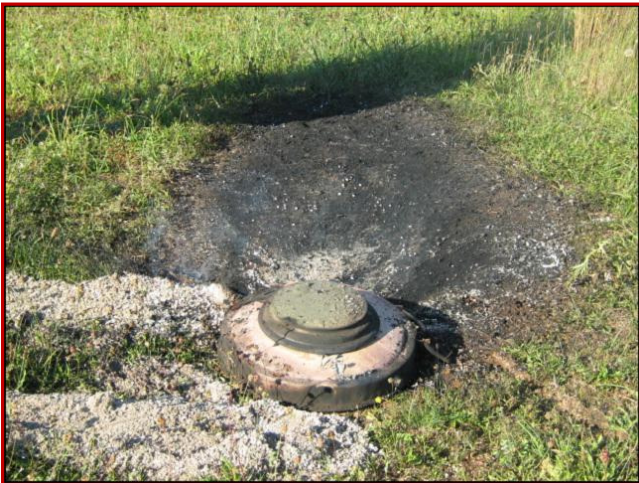
TMA-5 set up for burn
