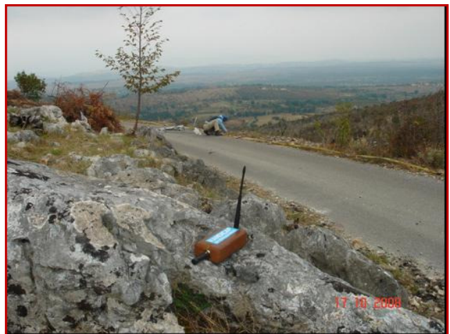
MineBurner set up showing repeater station
