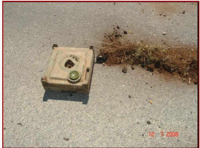
TMM-1 after MineBurner
