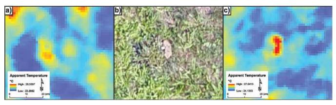
Figure 6. Apparent temperature from (a) 8:16-8:23 AM flight and (c) 9:18-9:24 AM flight before and after direct heating from sunlight, and (b) visible light color photos over the same area.
