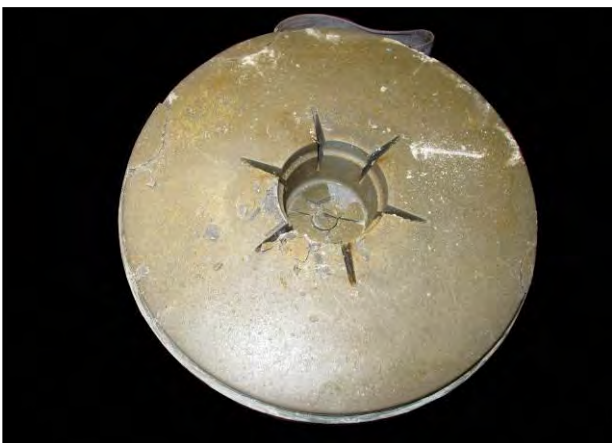
Figure A11 Upper section of the casing removed to reveal the main charge; most were in good condition with little or no cracking or deterioration evident in the explosive. Although the inside of the plastic casing was wet, the cast filling contains very few voids
