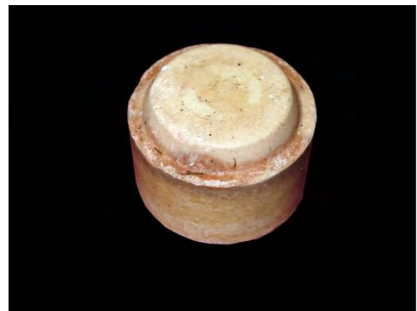
Figure A12 Booster pellets are composed of a pressed TNT/RDX (60/40) mixture and virtually all were in good condition. Despite the neoprene seal between the base of the fuze and the booster, all of the booster pockets contained water
