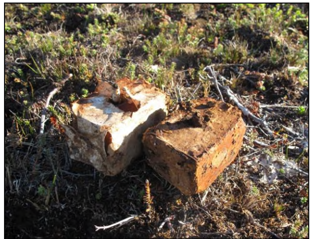
Figure C5 TNT blocks containing detonators and the remnants of safety fuzes. It is clear that any pyrotechnic composition in the fuse or detonator will be non-functional. However, findings from the Ageing Study (involving explosives of a similar type and age) suggested that the primary explosive in the detonator may be viable; this means that the explosive could be initiated by either fire or substantial impact
