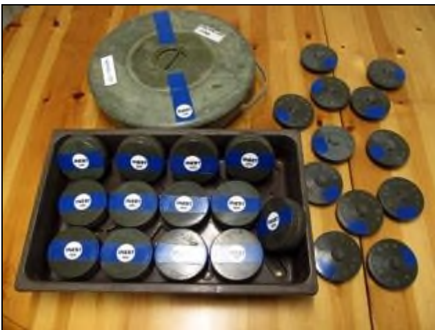
Figure 5: Inert Spanish P4B AP mines, with the wax-filled C3B body to the top left
