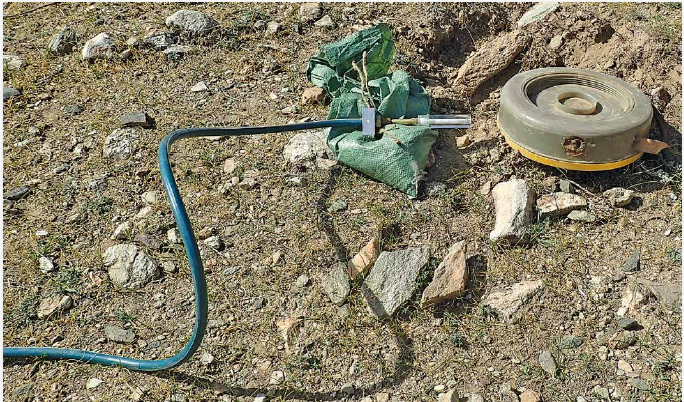
Figure 8. Test setup using the HTL to destroy a Pakistani P3 Mk2 anti-tank mine. Figure courtesy of Donald Pratt.
