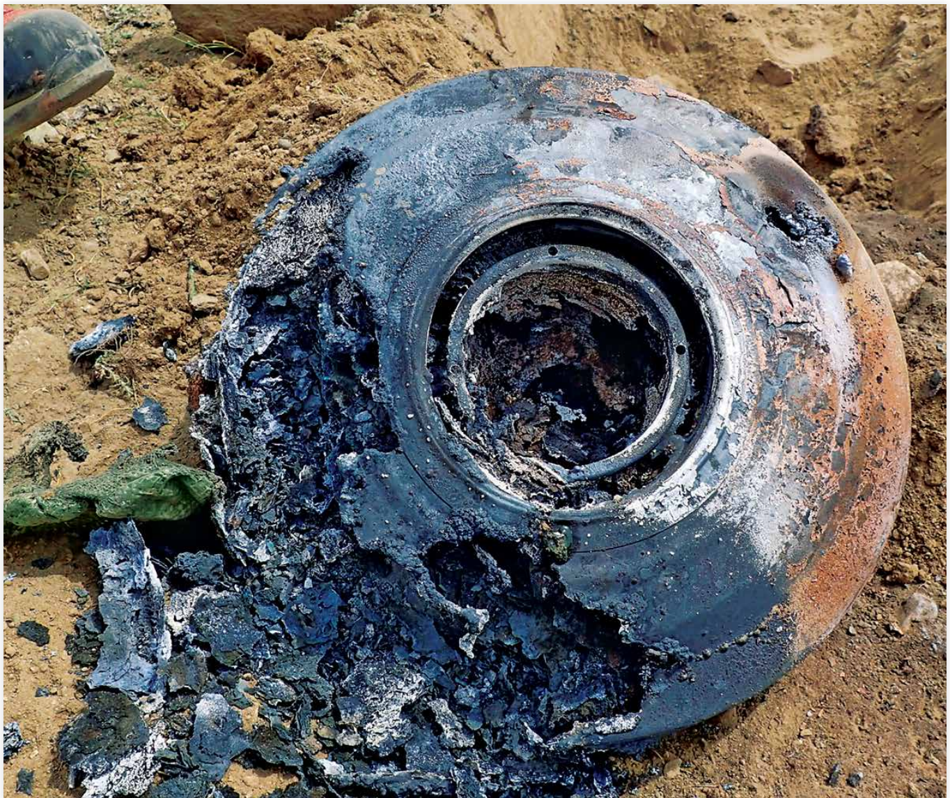
Figure 13. Remnants of the TM-62M anti-tank mine after exposure to the HTL. Figure courtesy of Donald Pratt.
