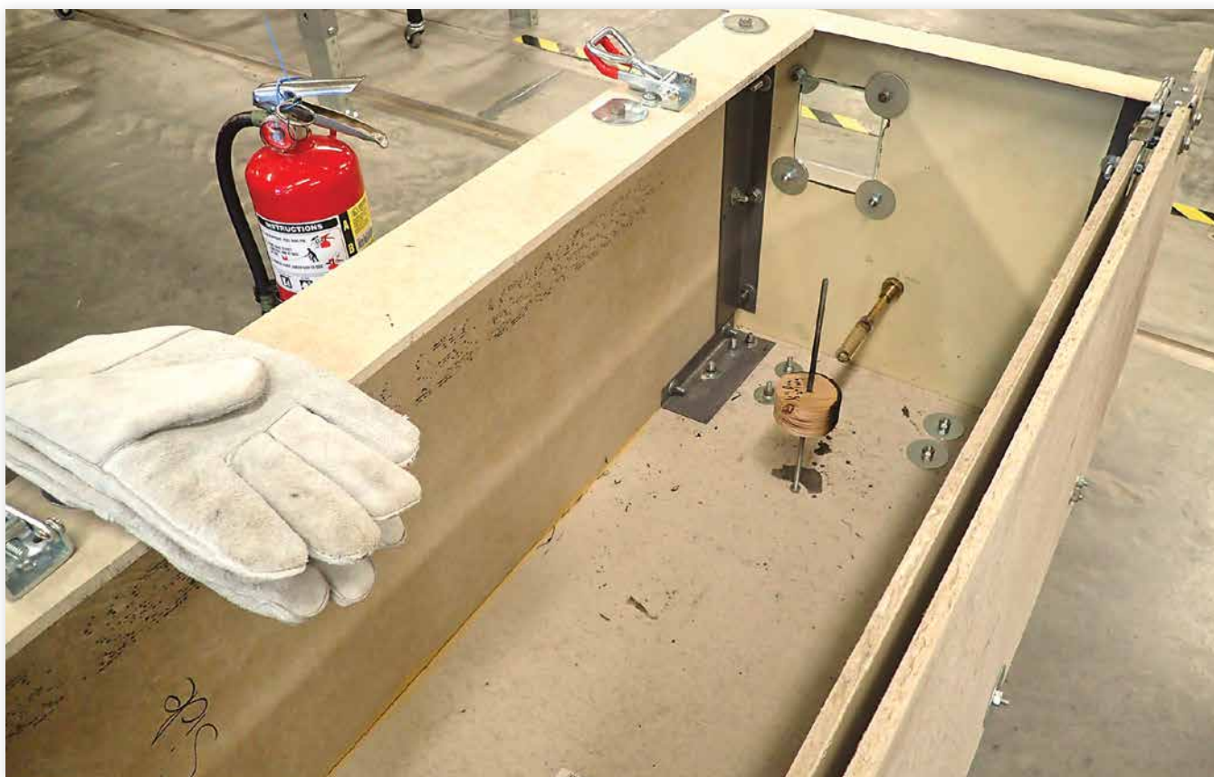
Figure 3. Fireproof test chamber used for initial prototype testing in the laboratory. Figure courtesy of Donald Pratt.
