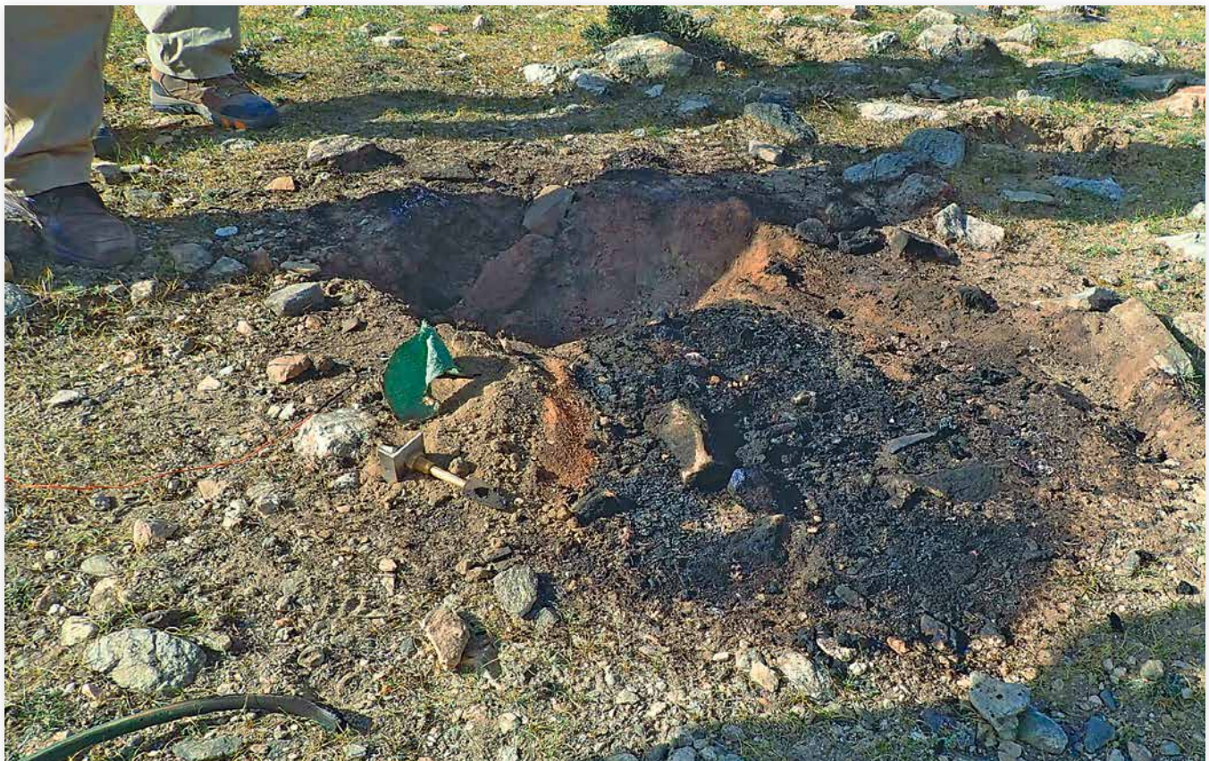
Figure 9. Nothing remained of the P3 Mk2 anti-tank mine after exposure to the HTL. Figure courtesy of Donald Pratt.
