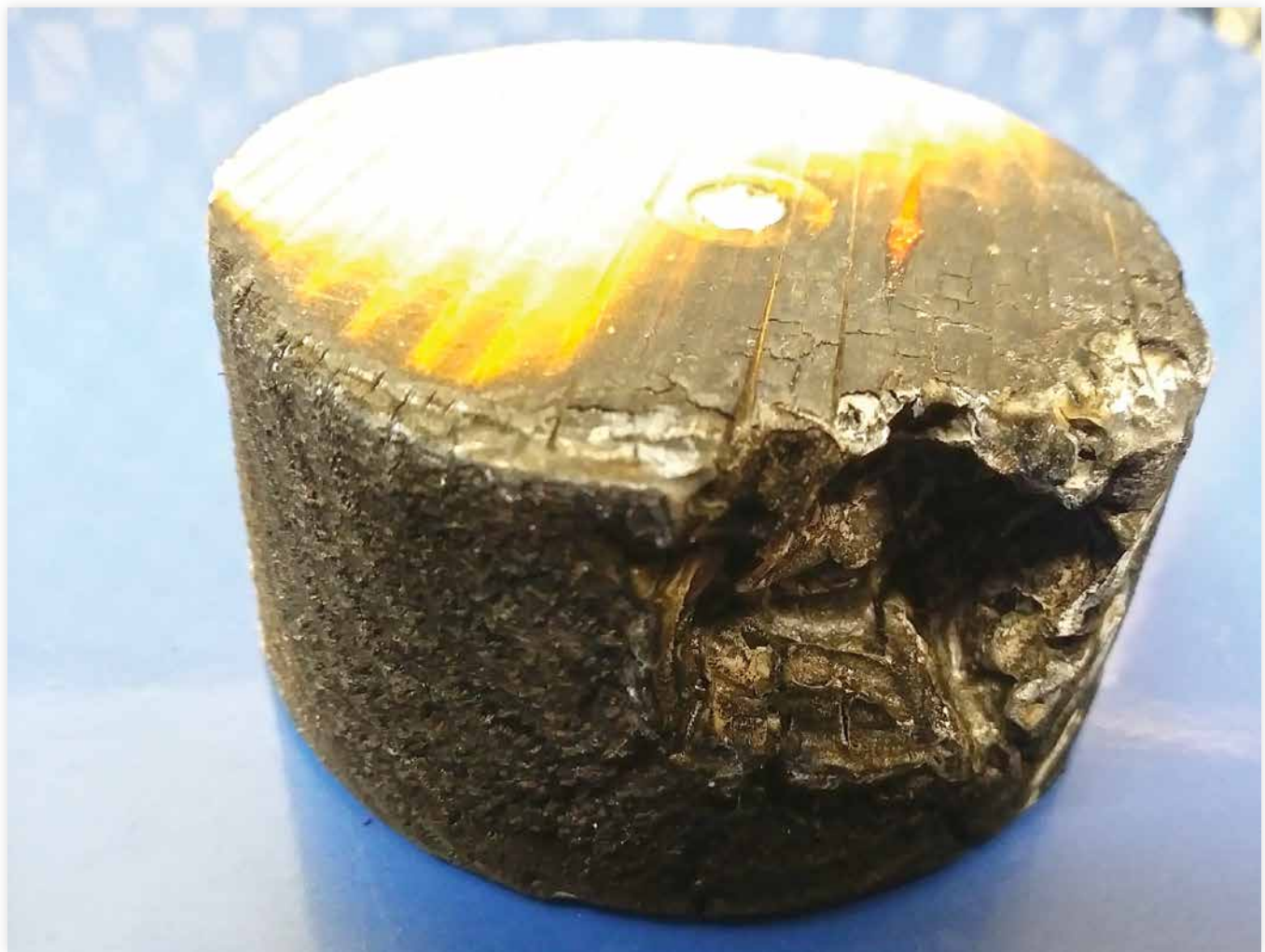
Figure 5. 3" diameter wood test sample after 20 second exposure to the HTL. Figure courtesy of Donald Pratt.
