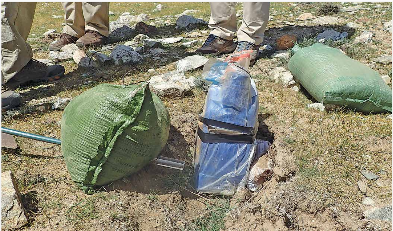
Figure 6: Test setup using the HTL to destroy a simulated IED explosive charge (loose-fill ammonium nitrate-based explosives). Figure courtesy of Donald Pratt.
