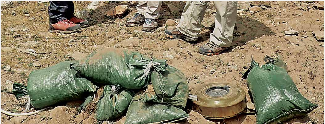
Figure 12. Test setup using the HTL to destroy a Soviet TM-62M anti-tank mine. Figure courtesy of Donald Pratt.
