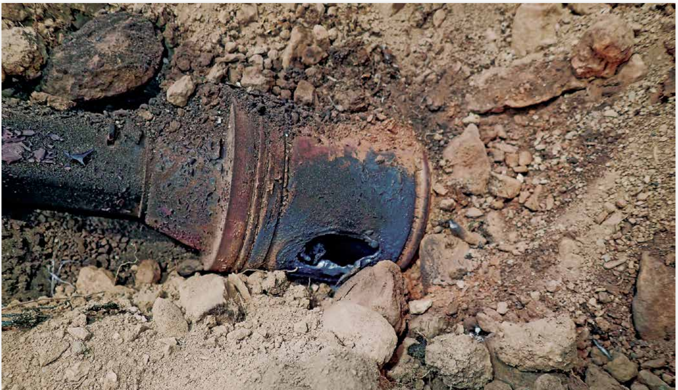
Figure 11. Penetration of the casing of the PG-2 grenade by the HTL. Figure courtesy of Donald Pratt.
