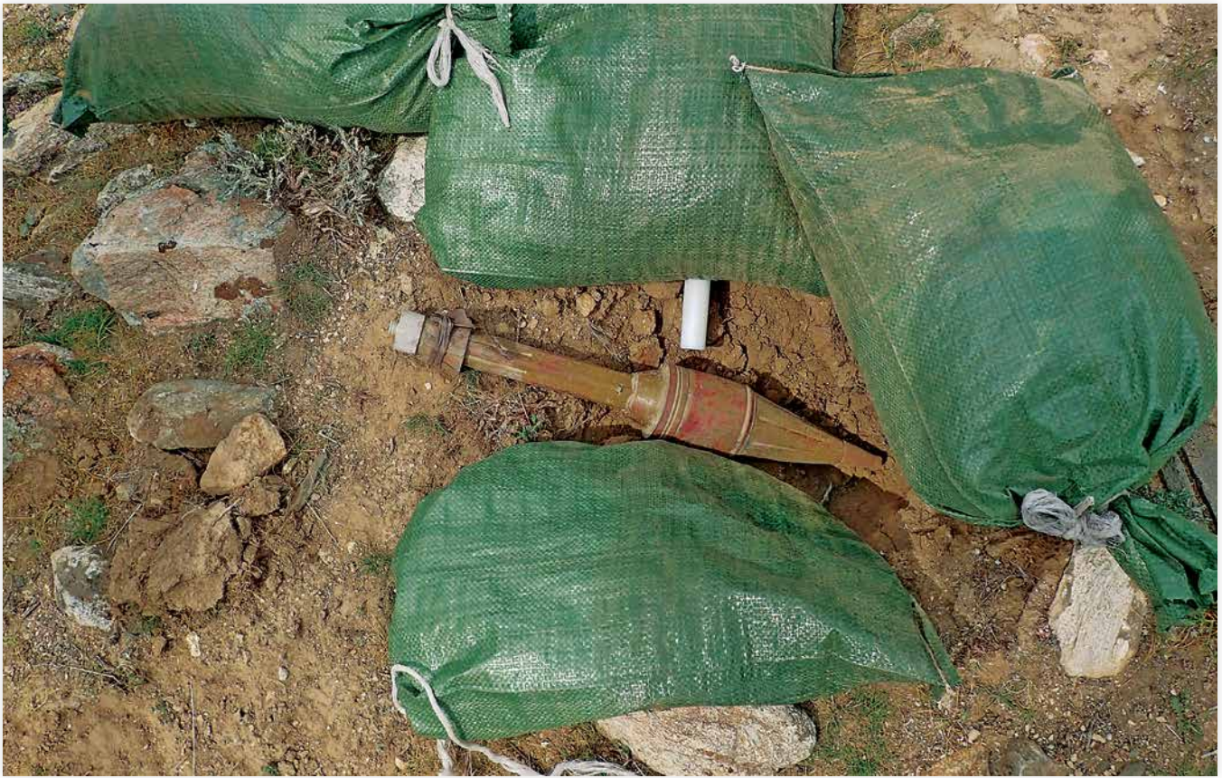
Figure 10. Test setup using the HTL to destroy a PG-2 grenade. Figure courtesy of Donald Pratt.
