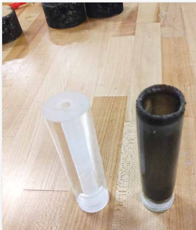
Figure 4. Prototype HTL fuel tubes made of 1" diameter 4" long PMMA before and after testing. Figure courtesy of Donald Pratt.
