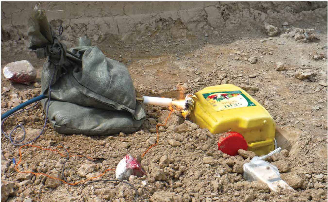
Figure 16. The HTL shortly after ignition burning through the plastic casing of a simulated IED explosive charge. Figure courtesy of John Montgomery.
