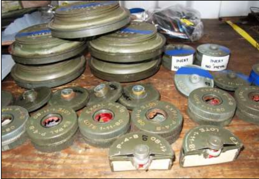
A number of inert training aids were produced, including sectioned P4B mines and inert mines, reconstructed with detectable detonator capsules
