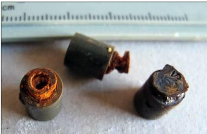
The spring in the P4B fuze is only detectable to a maximum of 5 cm, and many have rusted away
