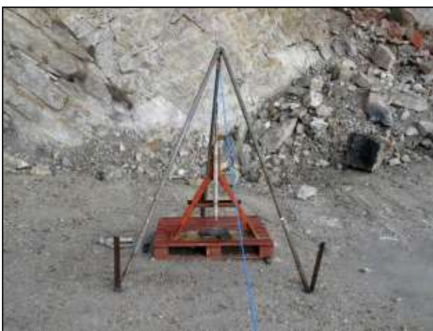
The explosive test rig used a rope and pulley to lower a steel rod onto the mine fuze
