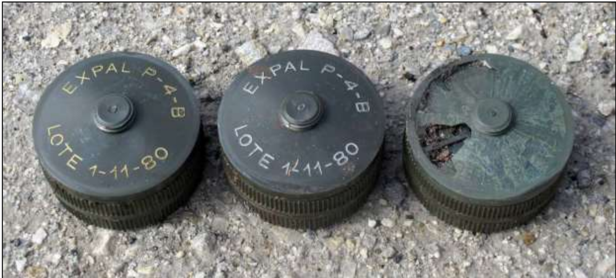
P4B mines from Lot 1-11-80 were found to be far more detectable than the types previously encountered. The variation in markings was also unusual for mines originating from the same batch.
