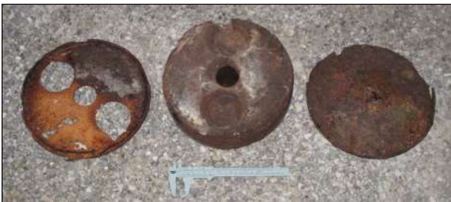
This mine was recovered during Phase 4. A brief examination concluded that it was an 'M1' and that, what at first appeared to be an inert filling, was in fact TNT. No fuze was present
