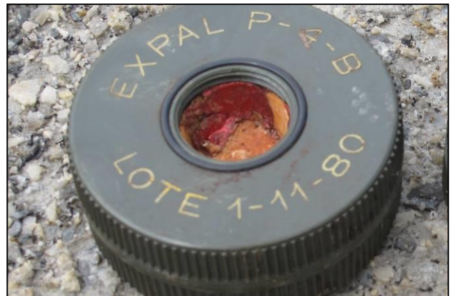
The red metallic foil is a lead/tin/antimony alloy and is virtually undetectable
