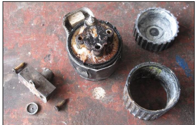
Examination quickly revealed the level of deterioration within the fuze mechanisms
