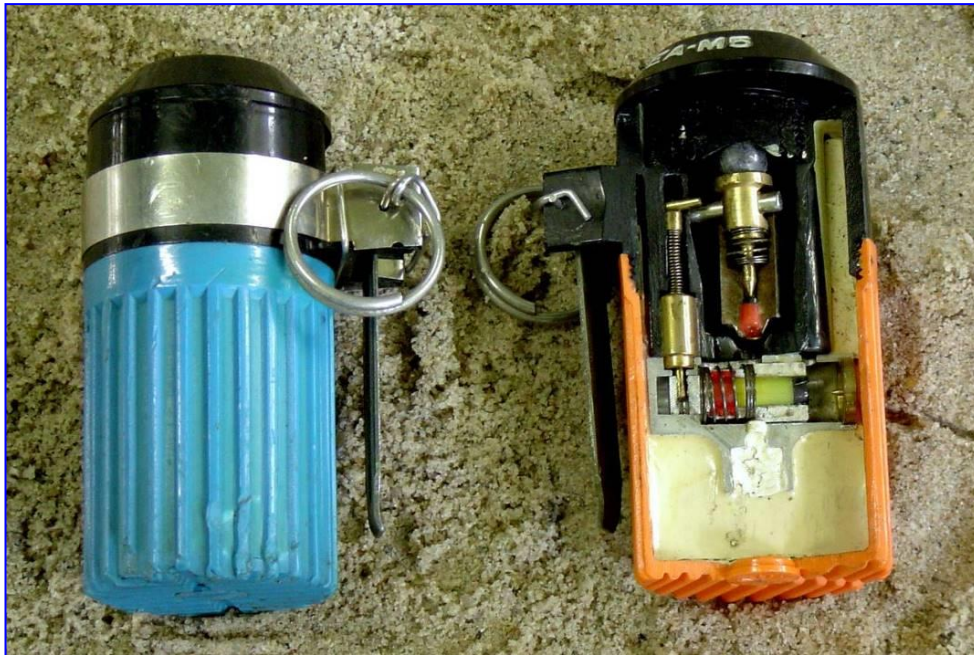
The Spanish M5 grenade. The lower casing of the live grenade is black
