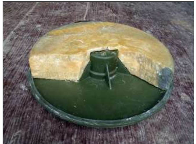
The distribution of aluminium within the explosive is very uneven; in some case, virtually absent
