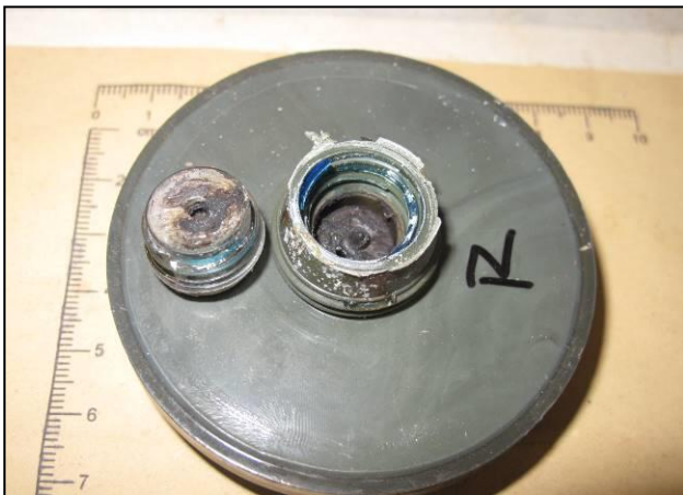
In two fuzes, only the stab receptor functioned, with the detonator failing to explode
