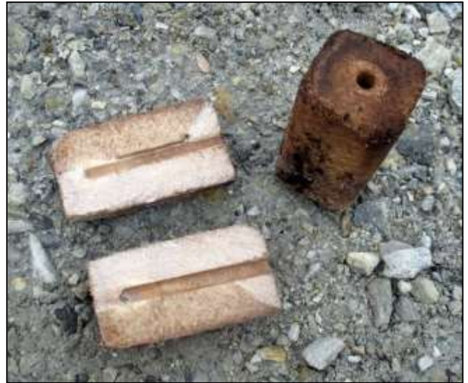
Internally, the explosive was still in good condition
