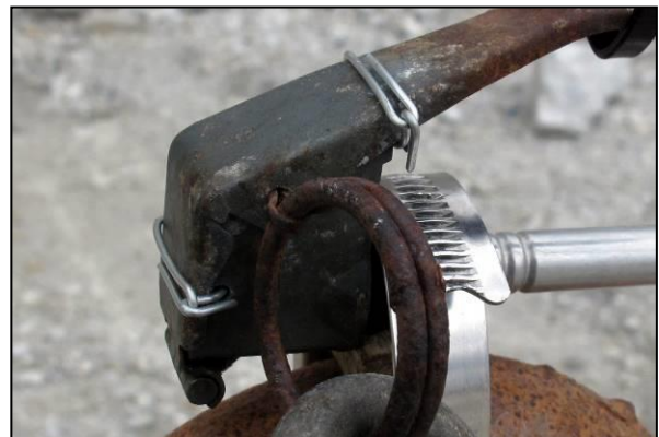
Safety wiring with the fly-off lever in place
