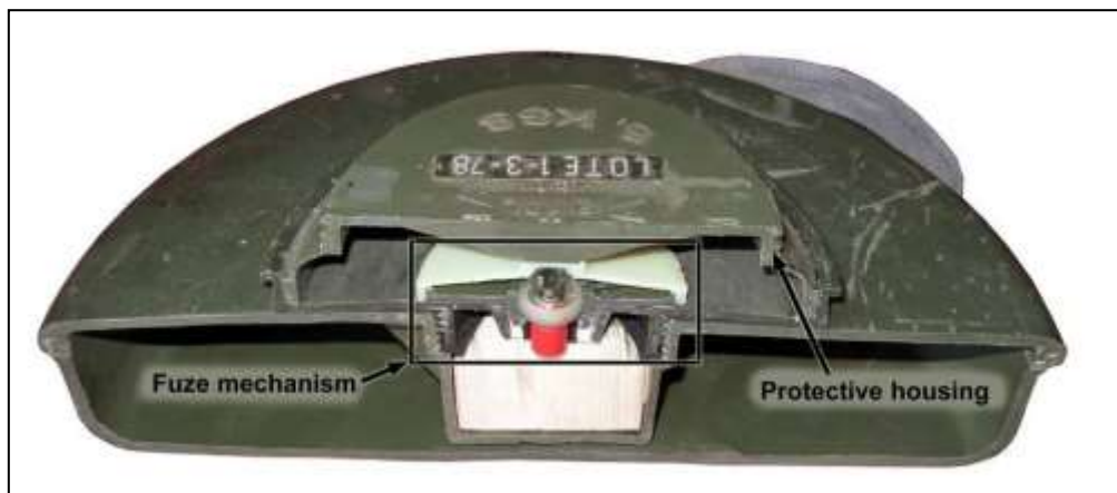
The protective housing of the C3B raises the operating pressure, but also helps to keep water out
