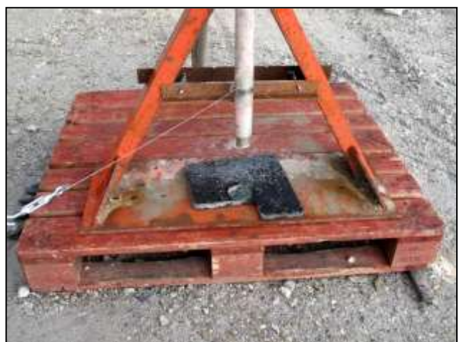
A P4B mine fuze placed on the test rig, ready for the rod to be dropped
