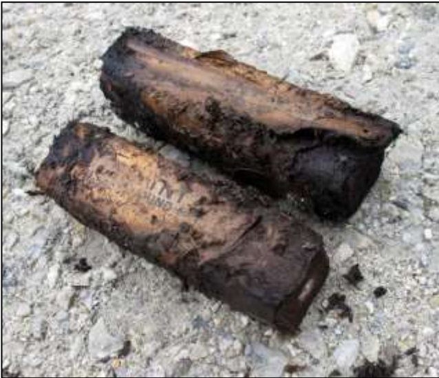
The TNT blocks appeared to be heavily degraded
