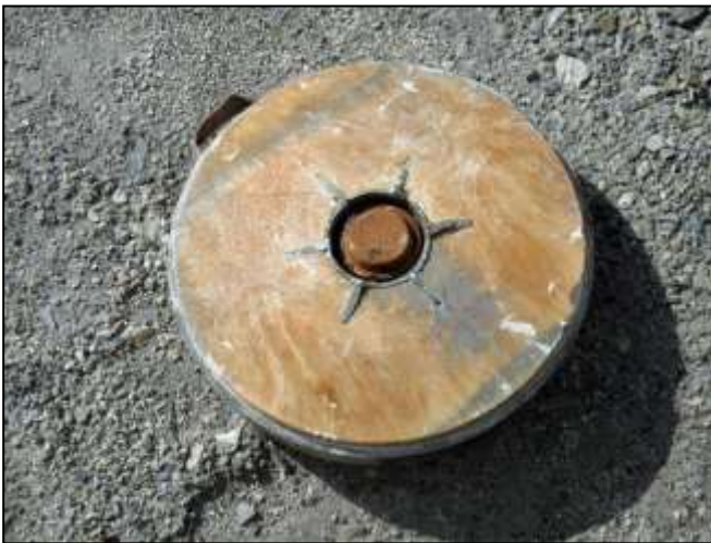
The central booster and main charge in C3B mines tend to remain in good condition
