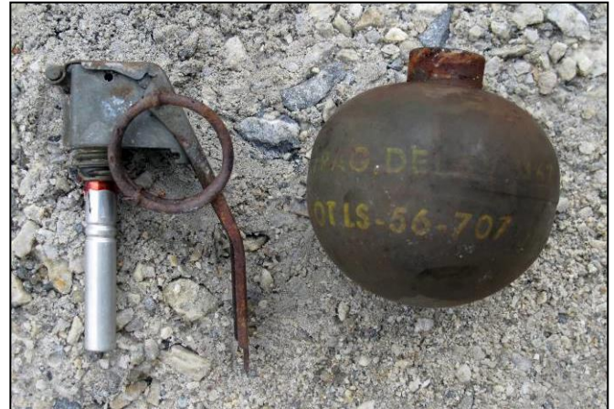
The fuze type and markings confirm that the grenade is indeed a US M67
