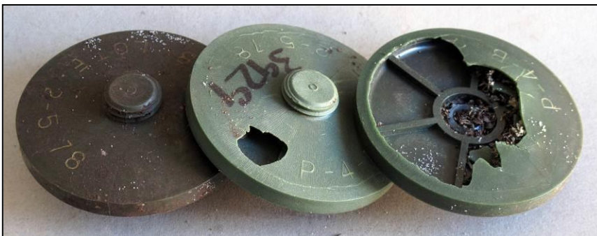
A range of degradation was present among P4B fuze casings
