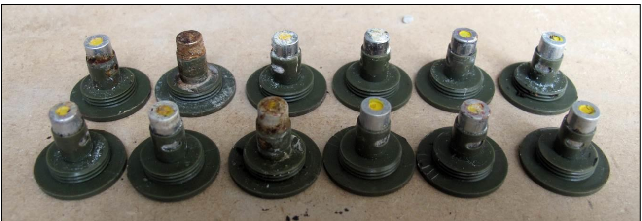
Detonators from the SB-81 mines, some of which show signs of deterioration
