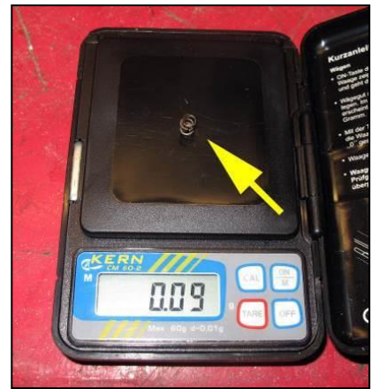
Figure A10 Due to corrosion, this striker Spring weighed only 0.09 g
