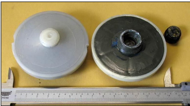
Figure A9 The sealed fuze assembly is very similar to that used in the P4B anti-personnel mine. Water was found inside almost all of these units
