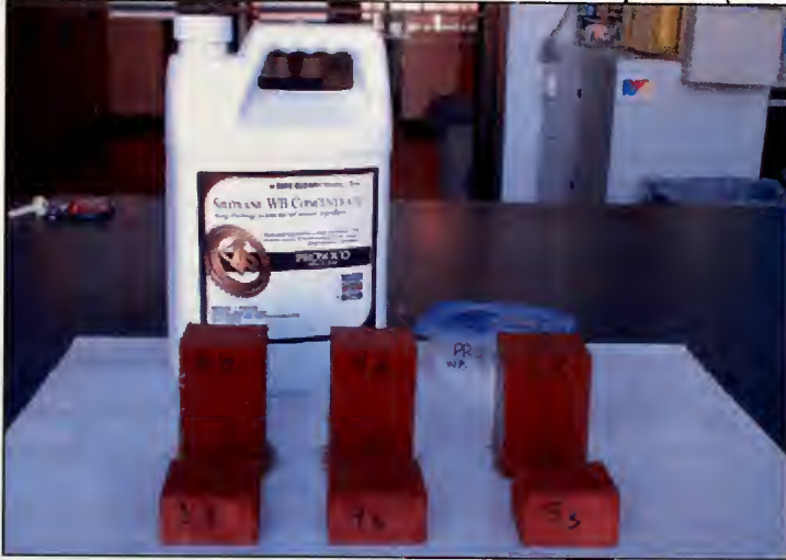
Sample Preparation Using Prosoco Siloxane WB Water Repellent
