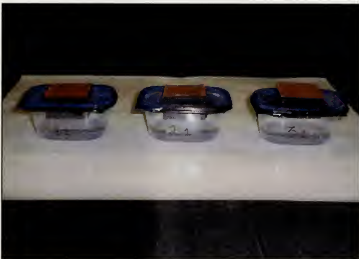
Prepared Samples in Containers for Water Vapor Permeability Test
