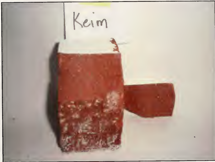
Salt Crystallization in Keim Granital Treated Samples
