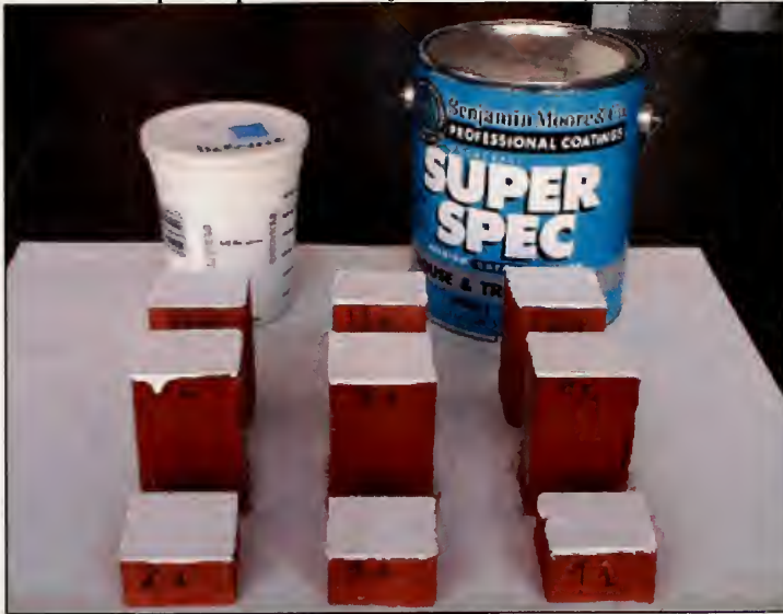
Sample Preparation Using High-Build Acrylic Masonry Primer and Superspec 100% Acrylic Exterior Masonry Coating
