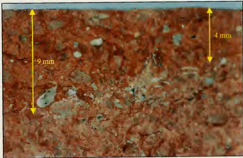
Salt Front of Prosoco Siloxane Treated Samples: Nikon SMZ-U Zoom 1:10 0.94x Magnification; 200 ASA
