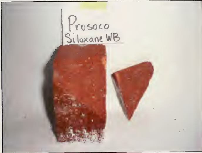
Salt Front of Prosoco Siloxane Treated Samples
