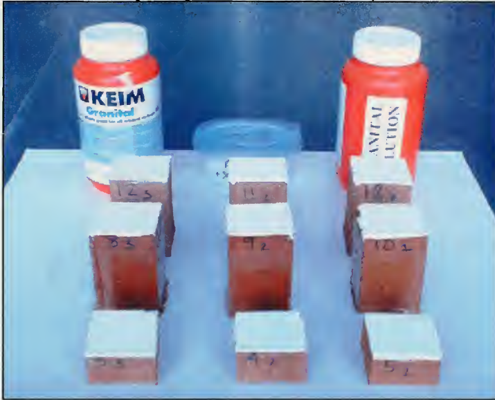
Sample Preparation Using Kiemfarben GmbH Granital with Keim Dilution Potassium Silicate System
