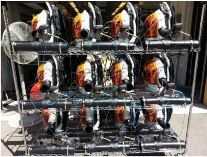
Figure 8-BR 600 STIHL mounted to aging rack
