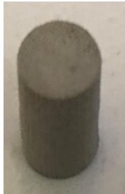
Figure 2.1-3: Binder jet additive manufactured solid cylindrical sample
