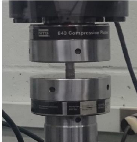
Figure 2.1-4: Sample in between compression platens of MTS Machine
