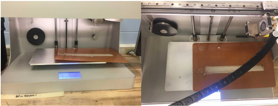
Figure 19 Failed print caused damage to print bed
