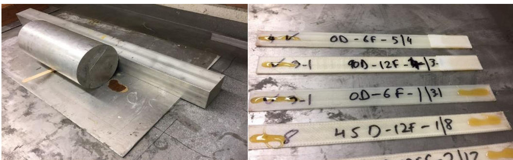
Figure 20 Attaching tabs to specimens
