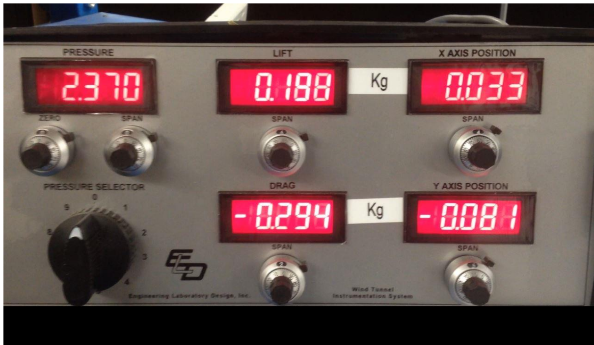
Figure 33. 10 Degree Wing Prototype Gauge Indication at 44.7m/s i.e. Test Wind Speed.
