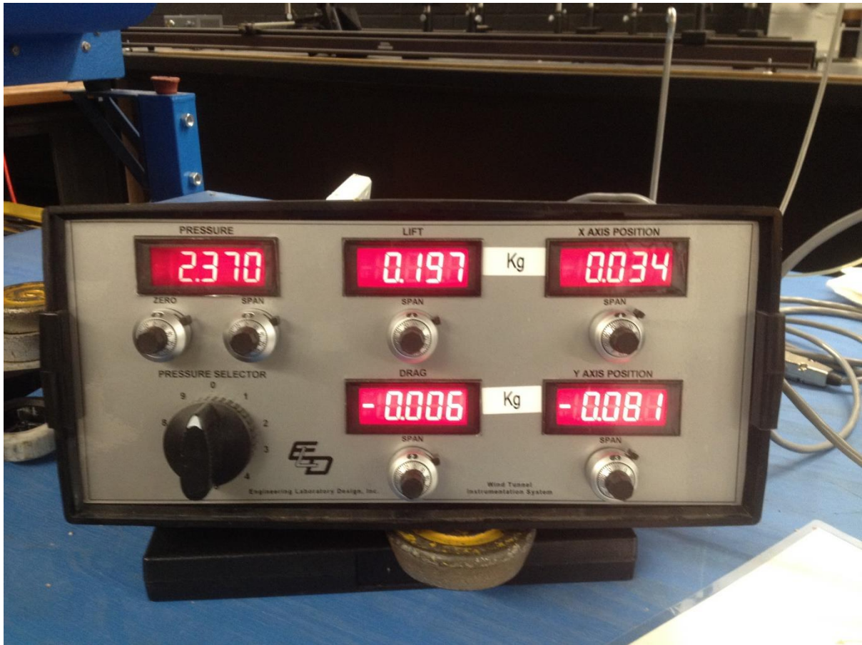
Figure 32. 10 Degree Wing Prototype Gauge Indication at Zero Wind Speed.
