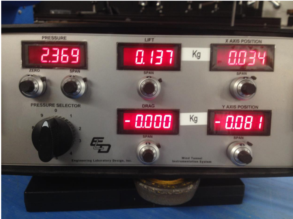
Figure 31. 0 Degree Wing Prototype Gauge Indication at Zero Wind Speed.
