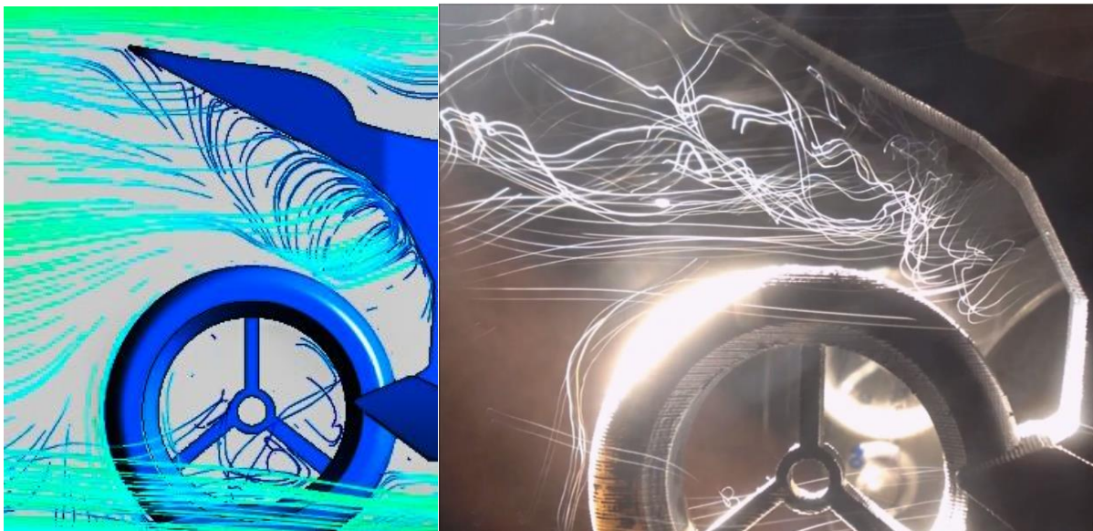
Figure 23. Validation of CFD Results: Vortices Formation under Tail Section and Streamlines behind the Wheel.
