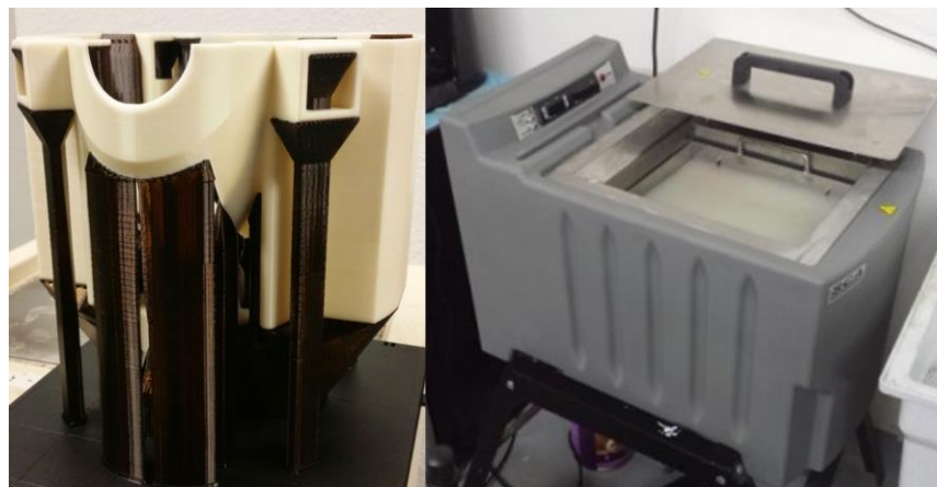
Figure 5.32: Left: Freshly printed part | Right: Heated chemical bath to remove soluble support structures
