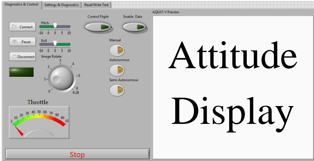
Figure 5.28: Ground Station Diagnostics and Control Page
