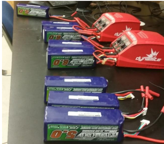
Figure 5.13: Chain of Nano-Tech LiPo Batteries being charged
