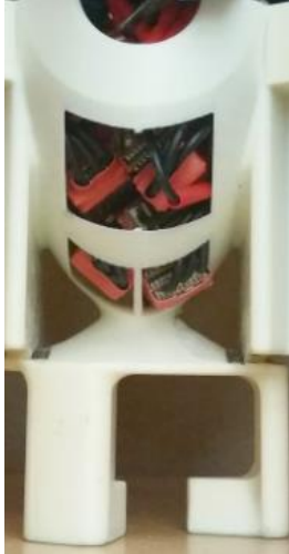
Figure 6.1: Congested cavity for V2
