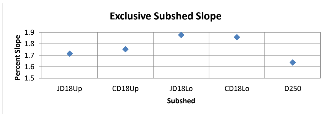
Figure 30. Slope percent per exclusive subsheds of the Lake Titlow watershed, McLeod and Sibley Counties, Minnesota. Exclusive refers to JD18Lo and CD18Lo not including their upland subsheds (JD18Up and CD18Up).
