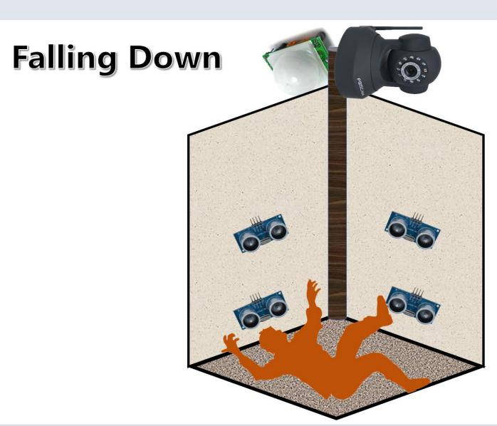
3) The adult has fallen down. In this case, only the two bottom ultrasonic sensors will detect the adult which means that the adult has fallen down. The system considers a possibility that an accident has occurred. At this time, the camera will be turned on.
