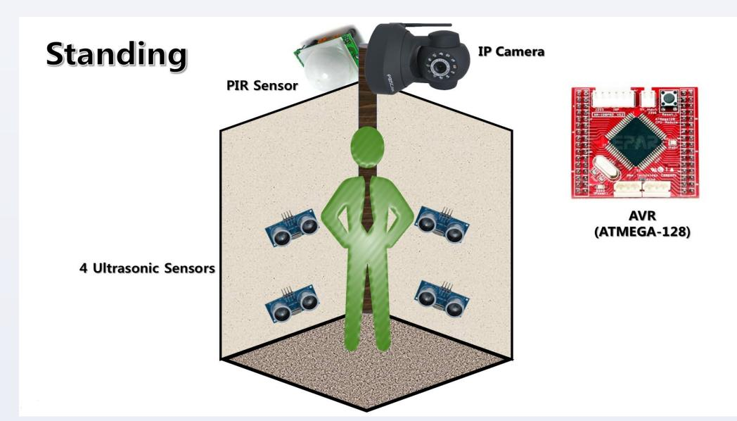
1) In this case, the adult is standing. First, the PIR sensor will detect the adult which means the adult is in the room. Then the four ultrasonic sensors will detect that the adult is standing. The IP camera will not be turned on because no accident has occurred.
