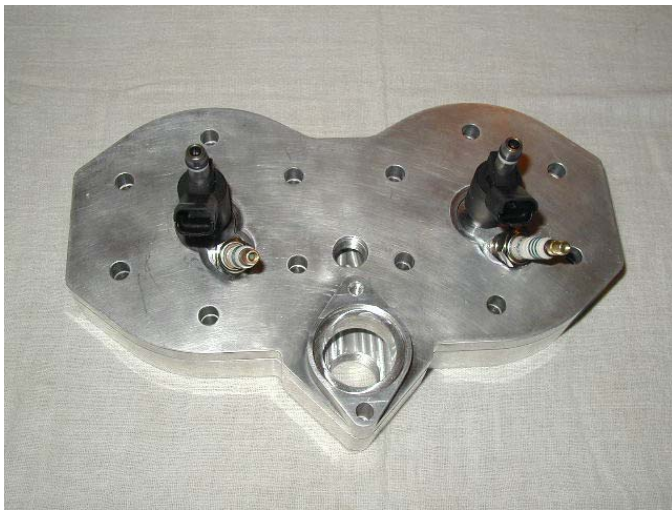
Figure 7: New Head, Spark Plugs, and Fuel Injectors
