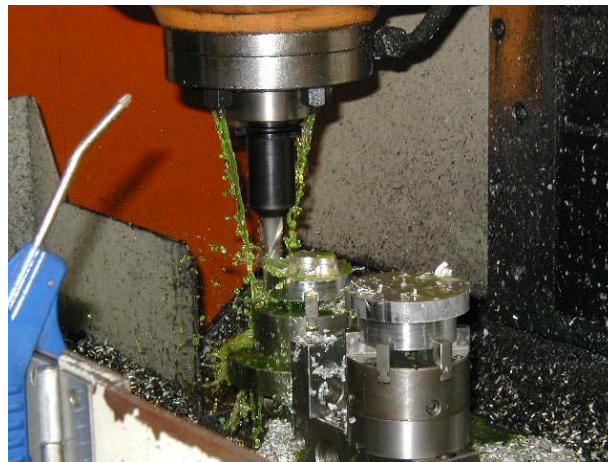
Figure 5: Machining of the Combustion Chamber
