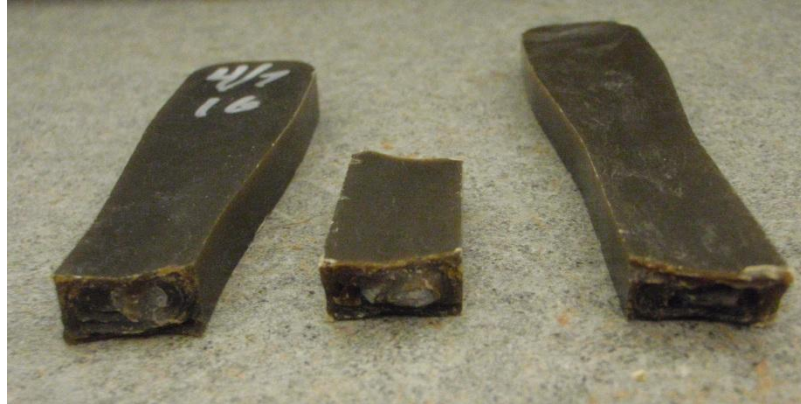
Figure 5: Specimen after Impact Test
