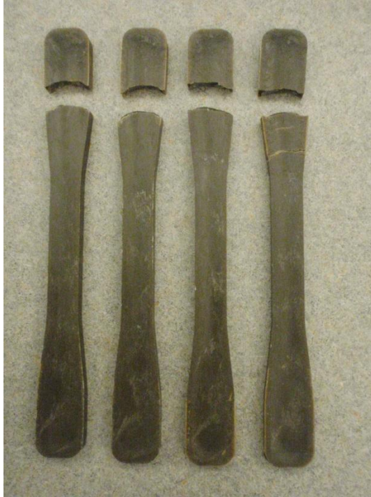
Figure 1: First Four Specimens after Tensile Test
