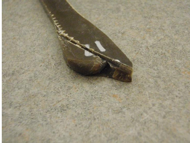
Figure 8: Partial Core Exposed After Attempting Diagonal Cut
