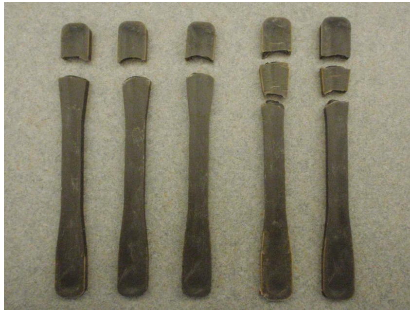
Figure 2: All Five Specimens after Tensile Test
