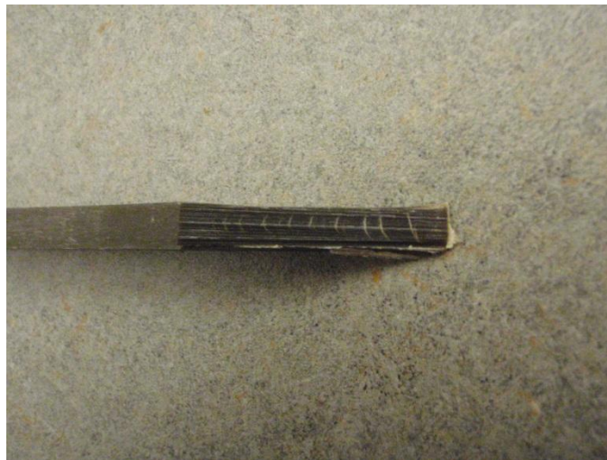
Figure 7: Specimen with end cut at Diagonal
