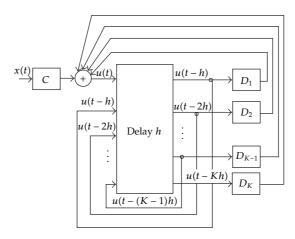
Figure 2: Implementation to enforce proportional delays.
