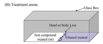
**Fig. 3.** Behavior bioassay test arena constructed on an open-top glass box  $(7.5\times7.5\times2.5~\text{cm}).$  (A) Control arena prepared with the ethanol (250  $\mu$ l) patch and the no-treatment patch. (B) Treatment arena prepared with the test compound-treated patch and ethanol-treated patch.
